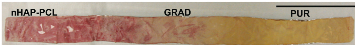
Figure 4.2: Photograph of Alizarin Red S-stained scaffold ES demonstrating the presence of a mineral gradient from the nHAP-PCL transitioning through the GRAD to the PUR region. Scale bar corresponds to 5 cm.
