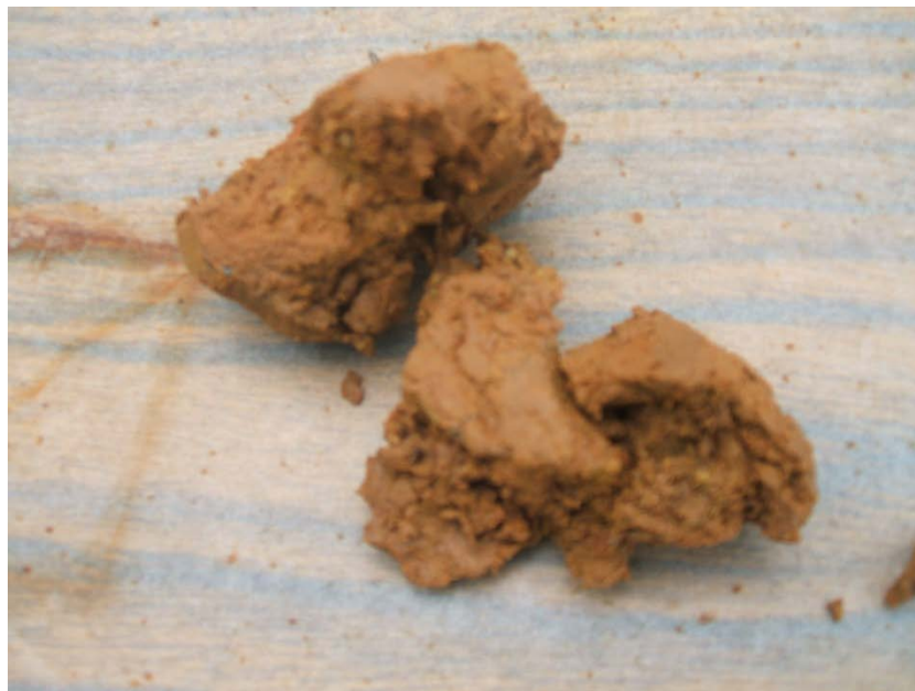
Figure 6.2. Soil cuttings taken while drilling the Test Pile hole.
