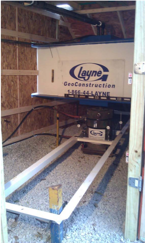
(d) Dial gauges and reference beam under the shed
