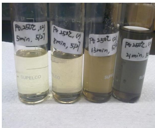
Figure 5.5: Color of chemical solution changed from light yellow to black as reaction time increases at 250°C.
