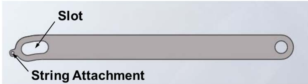
Figure 6.6: Slotted link ( L_{GH} ) for added passivity in Segment 3 during relaxation. The string attachment allows the link to regain its fully relaxed position as the rest of the arm relaxes.
