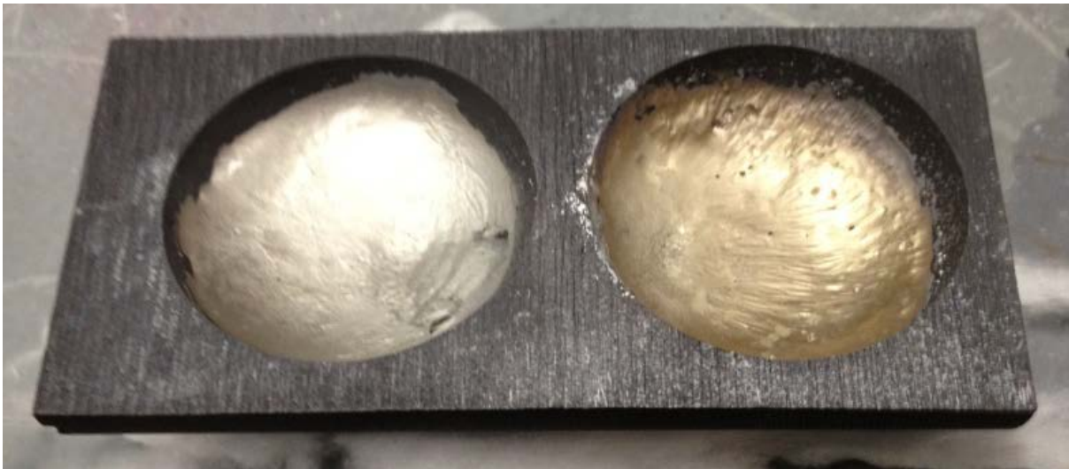
Figure 3.2.6: Crucible with melted samples. Left sample x = -4 , right sample x = +4 .
