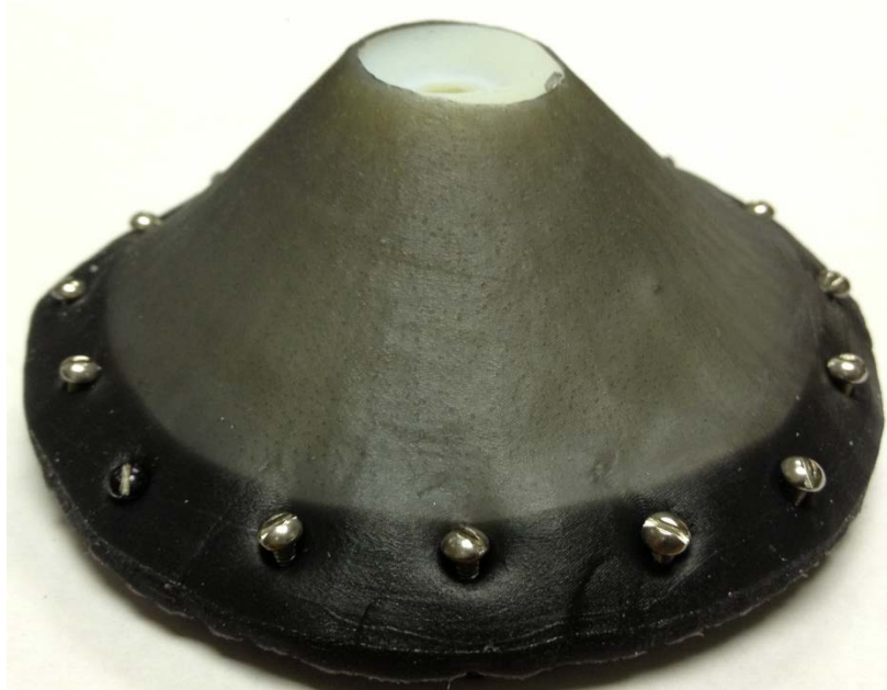
Figure 7.2.4: Constant cross section flap with angle of 45^\circ .
