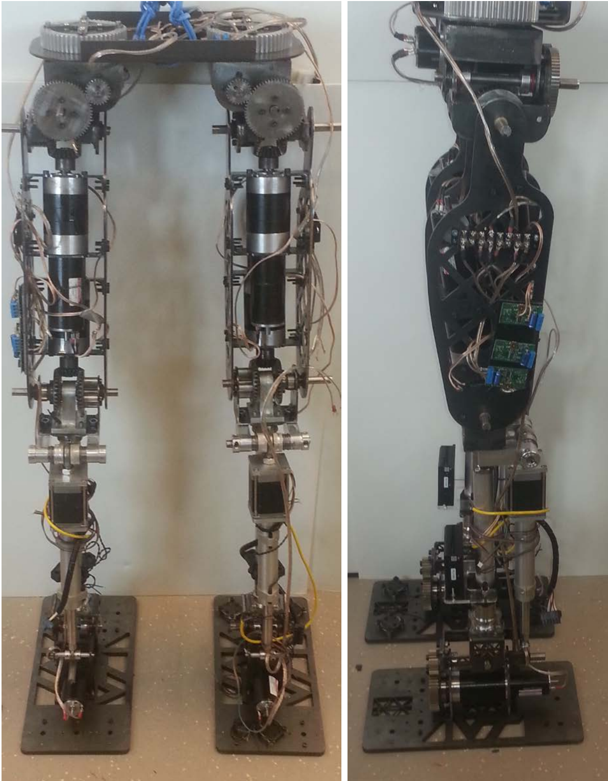
Figure 2.2.23. Final design from behind and from the left side. The electronics can be seen mounted to the outside of the hip plate on the right.
