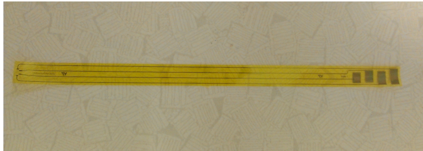
Figure 1.4: Fabricated bio-impedance sensor
