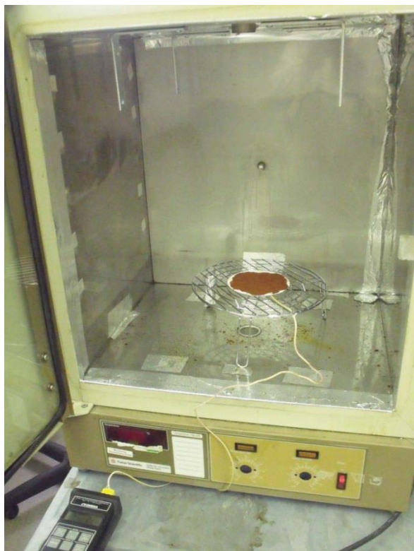
Figure 3.2. Ethanol treatment chamber showing a paprika sample on the sample holding rack. Note the 3/8" gas inlet on the back wall for application of vapor to chamber. The sample and filter paper rests on the thermocouple.
