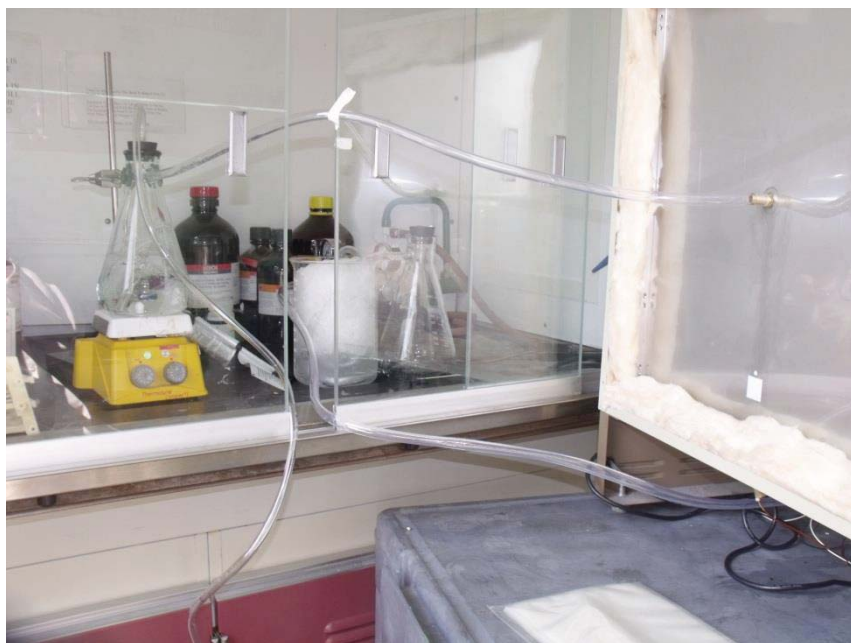
Figure 3.3 Tubing display for ethanol vapor delivery and condensation beaker for vapor withdrawal.
