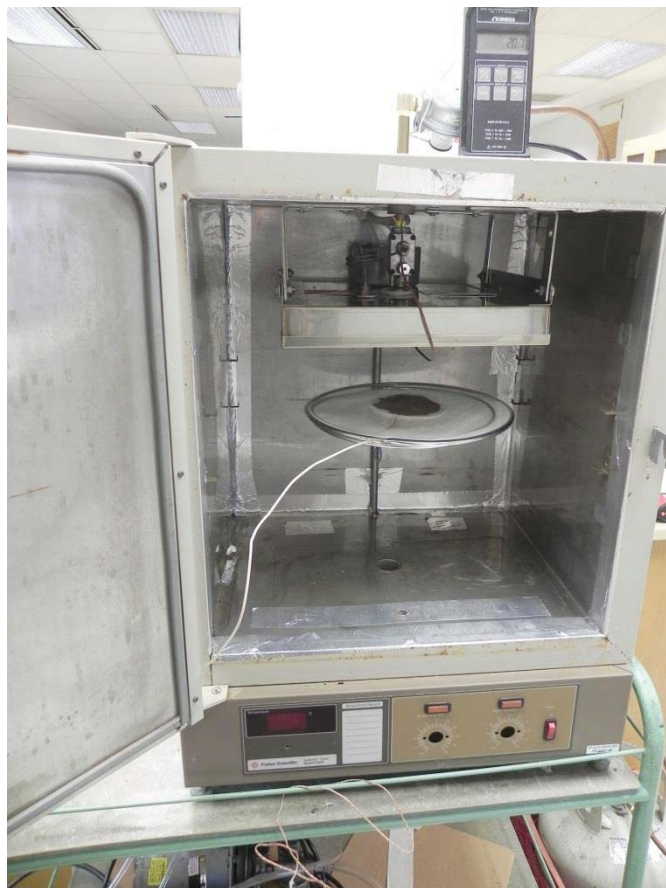
Figure 3.1. Far Infrared treatment chamber showing a black pepper sample in the four inch position on the sample holding rack. The sample tray was lowered from this position to the 6” and 8” treatment positions. The sample and filter paper rests on a thermocouple. The heater surface is also temperature monitored.
