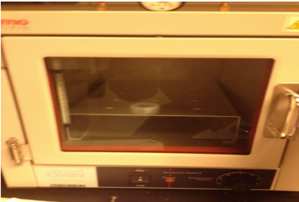
Figure 16 The oven and the container used can be seen. Although the container used in this experiment is larger than the "carrot", it is made of the same HDPE. (Photo by author)
