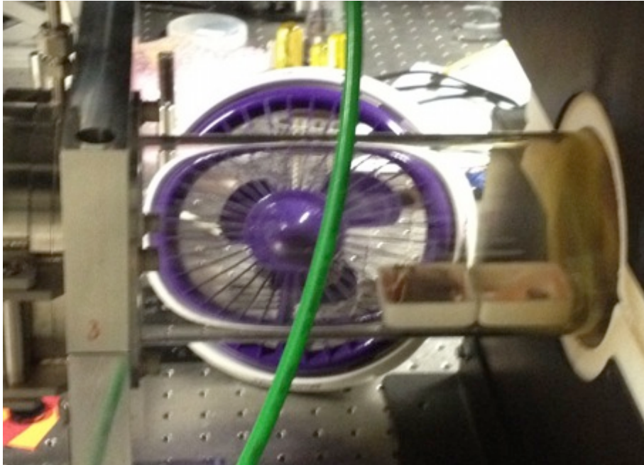
Figure 2 A CVD reactor shows graphene grown on a copper substrate. (Photo by author)
