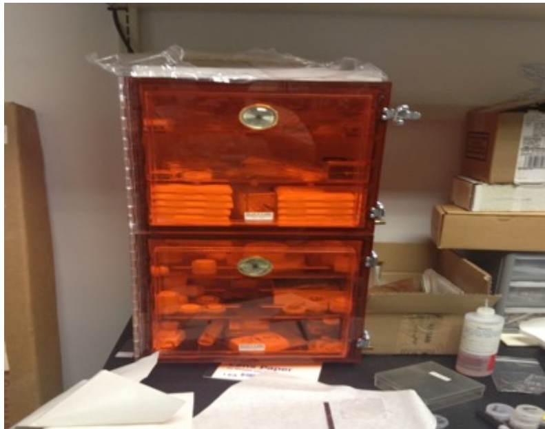
Figure 12 Shows an example of one of the vacuum boxes used to minimize the effects of ozone on the samples. (Photo by author)
