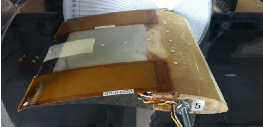
Figure 7: Selig S1210 high lift, low Reynolds number with 8541 MFC bimorph trailing edge
