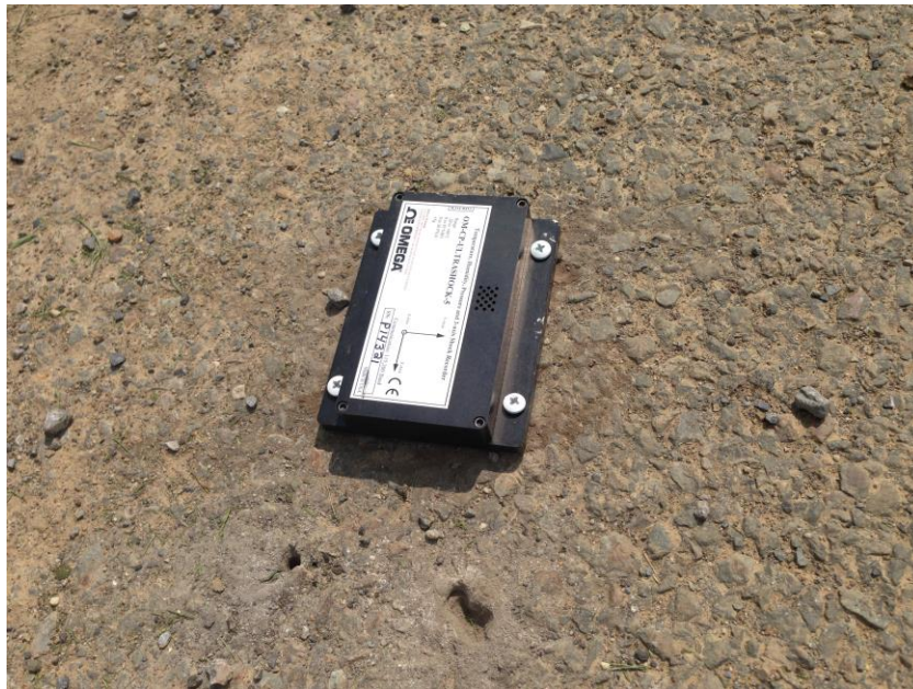
Figure 27 Sensor Installed on Pavement
