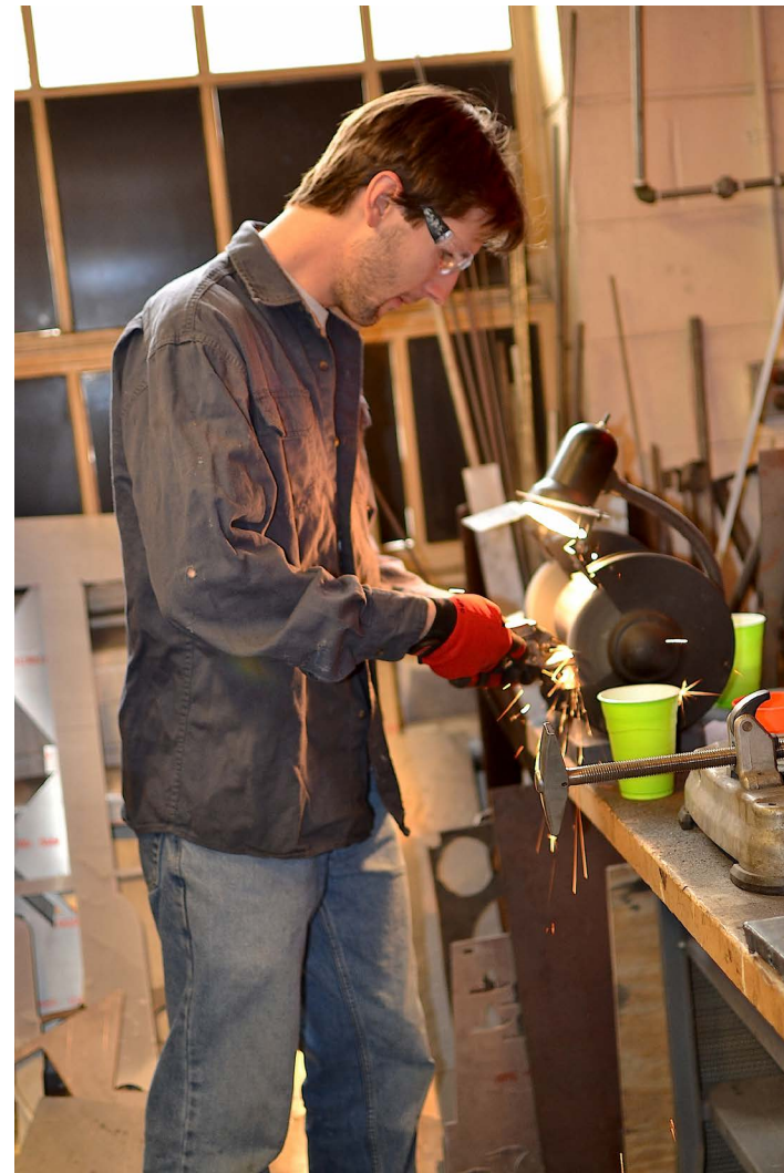
Formula SAE's Brian Oeters grinding a tab to be welded to the 2014 car's chassis in the Ware Lab.
