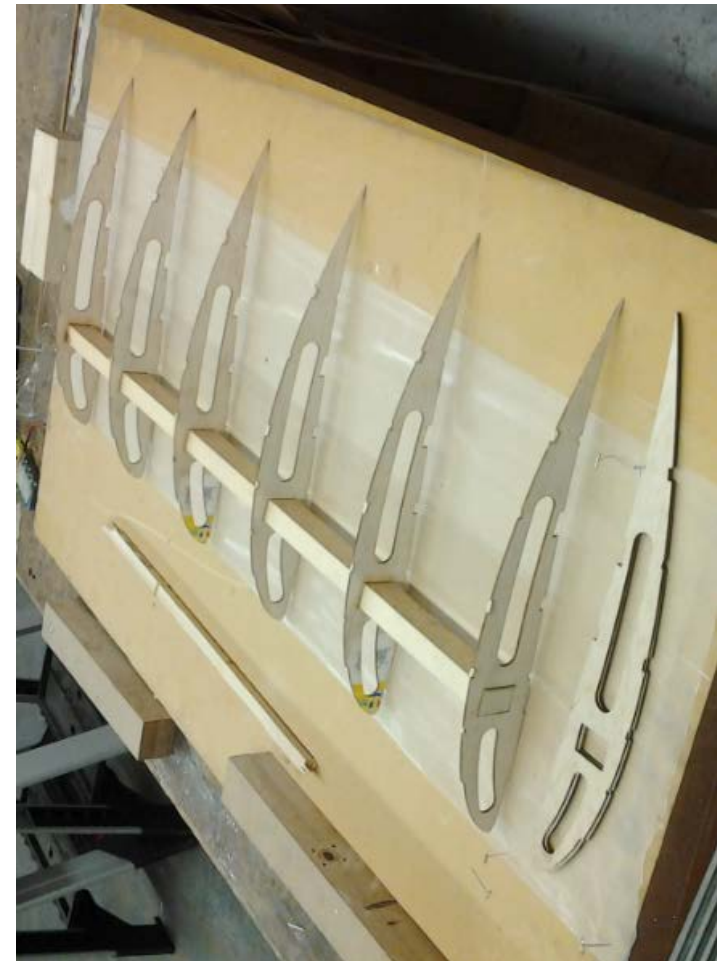
SAE Aero Design test wing under construction. Will be tested in a wind tunnel on campus to determine the theoretical lift coefficients of the team's wing design.
