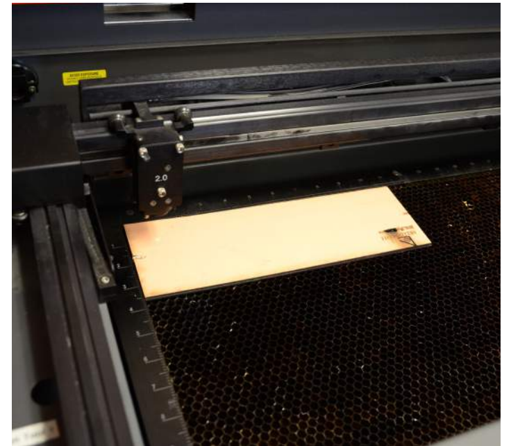
An inside view of the InVenTs Studio laser cutter while it is open and being calibrated to cut a design on the wood. The small red light seen in the upper left corner of the wood is the laser being positioned to cut in a precise location.
