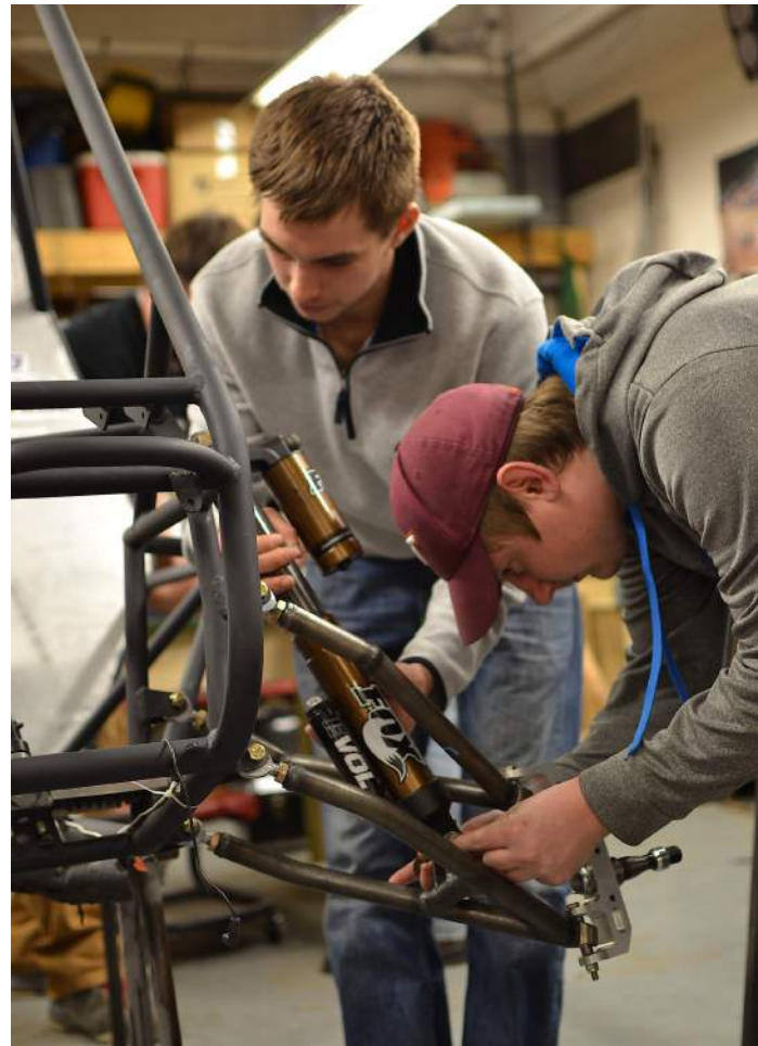
Baja SAE members hard at work connecting the shocks to the chassis above and the lower A-arm below.
