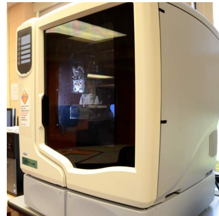
The InVenTs Studio 1 3D printer currently in process of printing a student's design.
