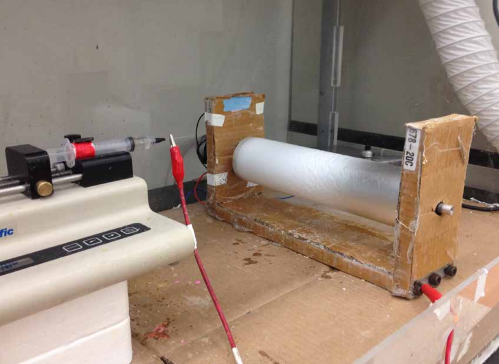
True electrospinning apparatus and setup. The white sheath on the aluminum foil is the collected microfibers.
