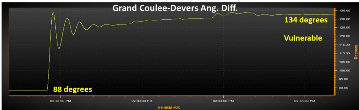
Fig. 6.21: RTDMS snapshot of Grand Coulee-Devers Angle Difference for outage of two PV units in a medium loaded condition
