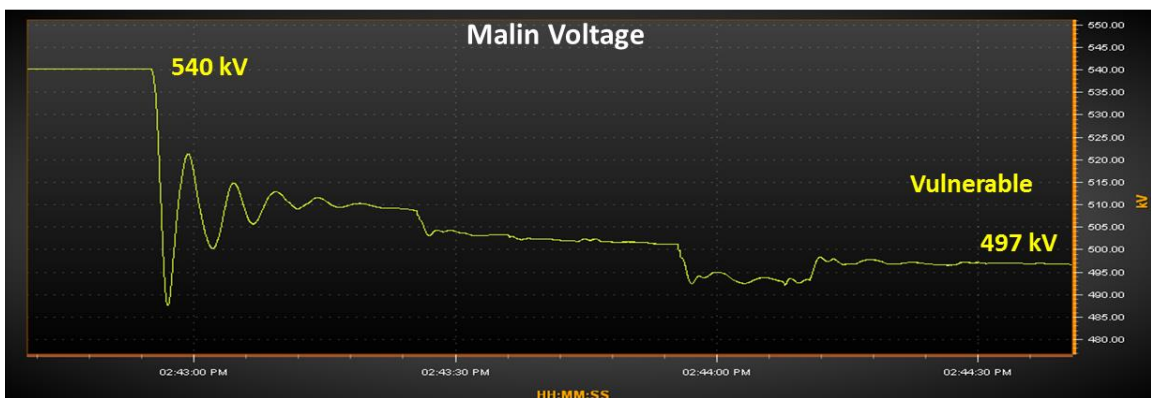
Fig. 6.22: RTDMS snapshot of 500kV Malin Voltage for outage of two PV units in a medium loaded condition
