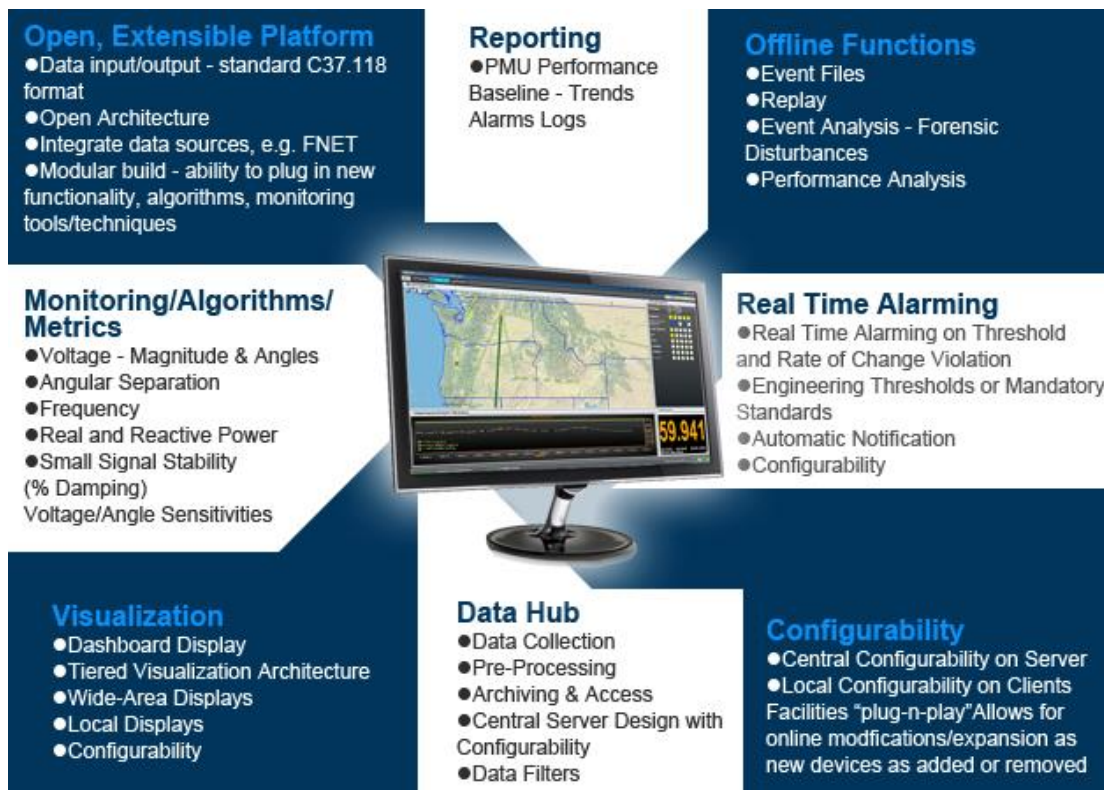
Fig. 6.18: RTDMS building blocks and functionalities
