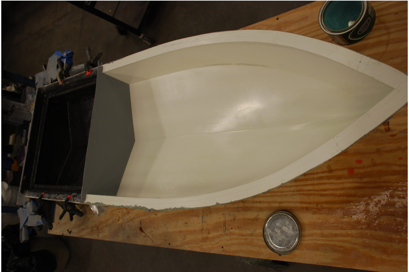
Figure 2.4: Afterbody Built in Mold
