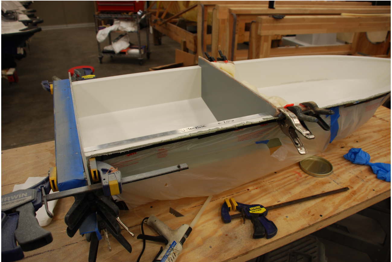
Figure 2.3: Temporary Dam Moved Forward 20 inches
