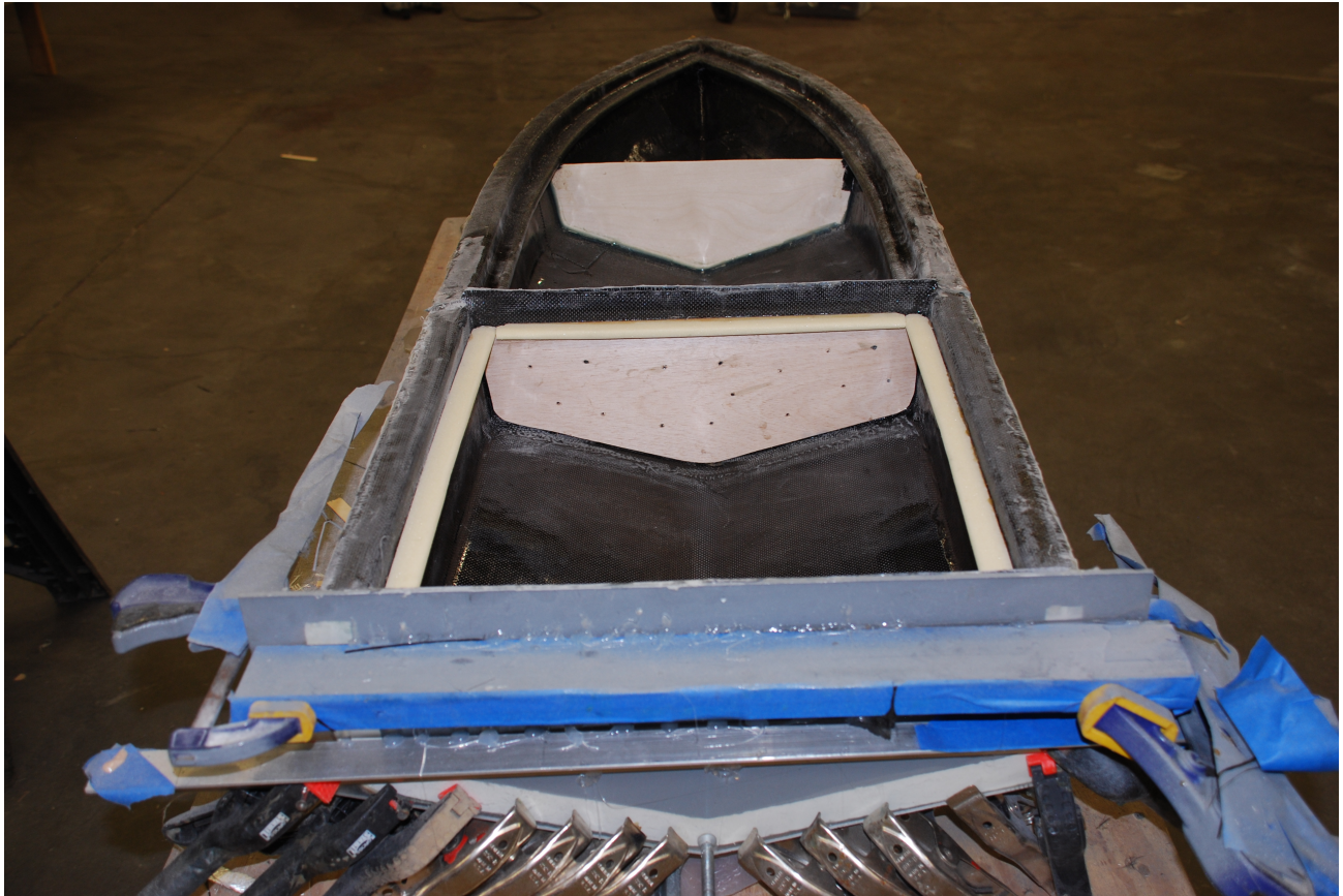
Figure 2.6: Midbody Construction: Before layup of Stiffeners
