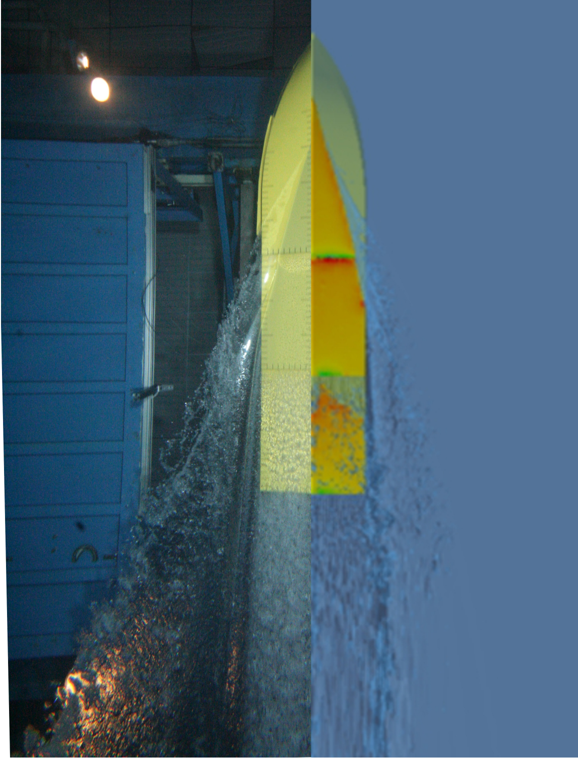
Figure 4.14: Comparison of Underwater Photograph to Simulation: Configuration 4, \Delta=85 lbf, C_v = 4.46 and LCG=40\% Forward of the Transom. Simulation captures overall wave profile. Simulation does capture fine spray sheet and stagnation line crossing step. Separation not predicted for forward step and the separated flow on the aft planing surface looks similar.
