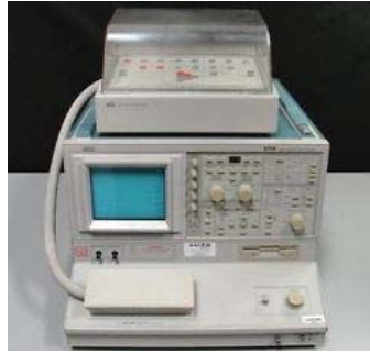
Figure 5-14. Curve tracer (Tektronix 371A) for the breakdown voltage and I-V curve measurement.
