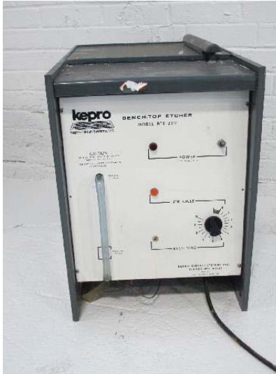
Figure B-7. Bench-top etching system from Kepro Circuit Systems (BTD-201B).
