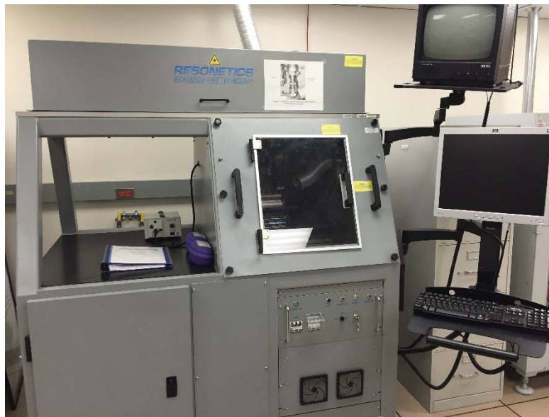
Figure B-6. Laser routing system from Resonetics Micromachining.
