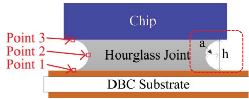
Figure 3-3. Illustration of the hourglass joint with defined geometry factor ( GF=h/a ).
