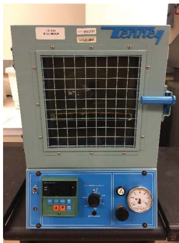
Figure B-9. Pressure-controlled environment chamber from Tenney for curing molding compounds.
