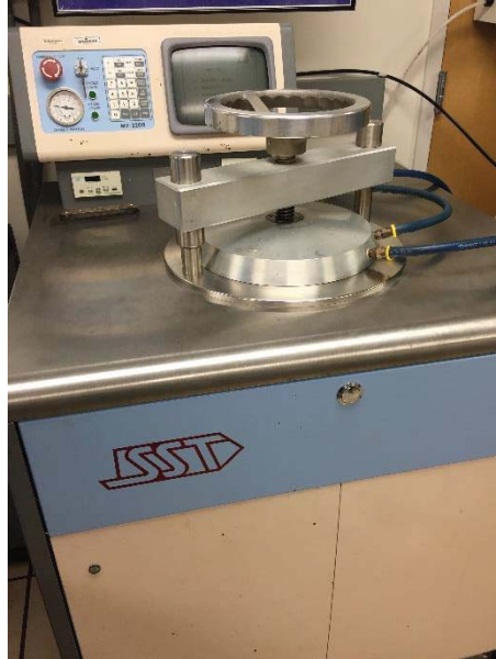
Figure B-8. Vacuum reflow chamber from SST (MV2200).
