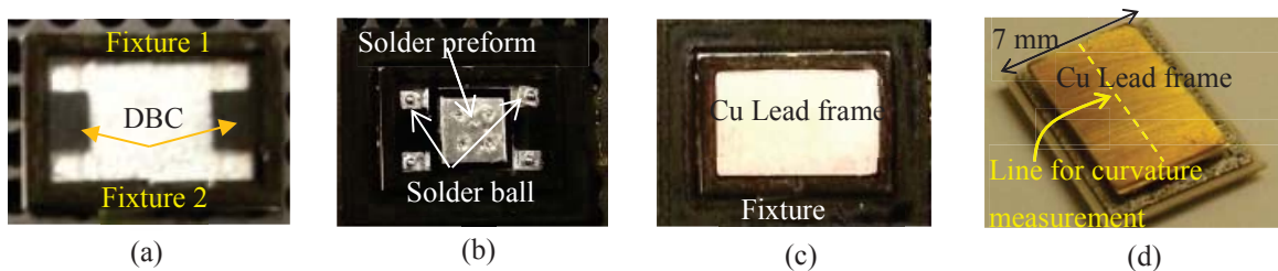
Figure 4-15. Fabrication process of the samples for curvature measurement (the same dimensions in Table 4-2): (a) DBC substrate with fixtures; (b) solder balls and preforms; (c) Ni-Au-coated copper lead frame; and (d) packaged module after solder reflow (see Appendix B.3 for the material fabrications).
