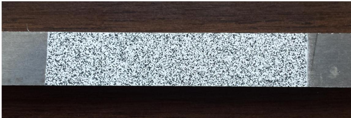
Fig. 17 Paint pattern for DIC test sample
