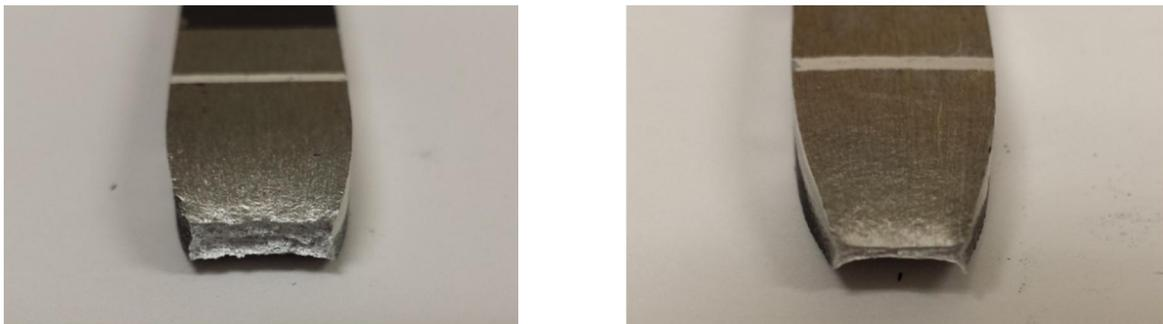
Fig. 29 Fracture surface of thermo-mechanical tested samples (a) 300°C, (b) 400°C
