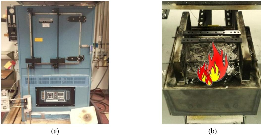
Fig. 2. Heating equipment (a) Blue M Furnace (b) Sand Burner
