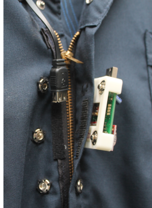
Figure 4.1: Snaps enable adjustment in a linear fashion along the primary axis of the limb segment
