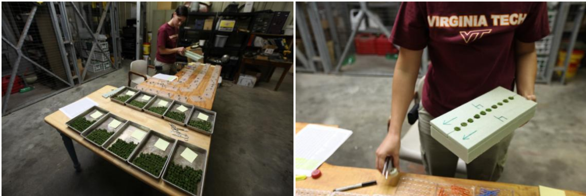
Image 2. Silvery threadmoss plugs sorted by replicate (left); and silvery threadmoss in a jig created to simulate spray coverage on a golf course putting green when sprayed in a spray chamber (right).
