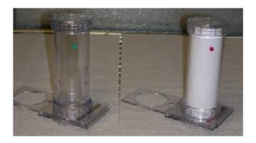
**Figure 3. 2.** WHO assay kit for testing carbamate chemicals on adult mosquitoes. The holding and treatment (exposure) chambers are on the left and right; respectively.
