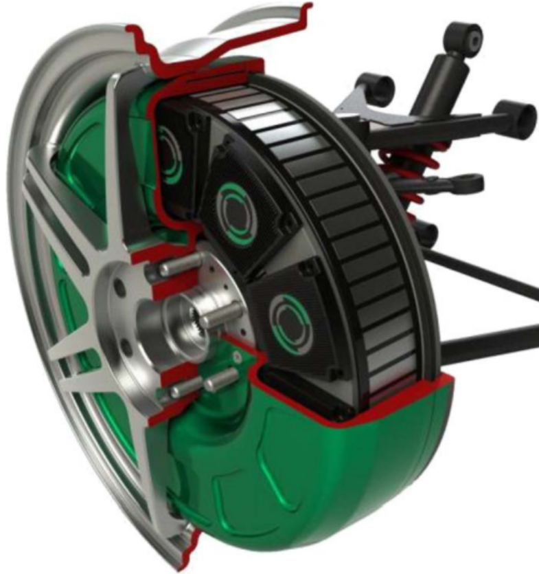
Figure 2.1: Design of a wheel hub motor for automotive use attached to a suspension, [5], C. J. Ifedi, B. C. Mecrow, S. T. M. Brockway, G. S. Boast, G. J. Atkinson, and D. Kostic-Perovic, “Fault-Tolerant In-Wheel Motor Topologies for High-Performance Electric Vehicles,” IEEE Transactions on Industry Applications , vol. 49, no. 3, pp. 1249–1257, May 2013. Used under fair use, 2014
