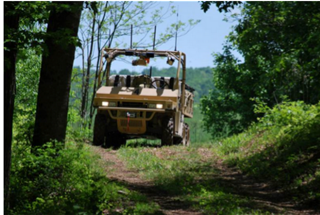
Figure 2.7: Ground Unmanned Support Surrogate utilizing the Polaris MVRS 700 6x6 platform, [11] Mechatronics Lab, “GUSS.” [Online]. Available: http://www.mechatronic.me.vt.edu/Projects/projectsPage.html Used under fair use, 2014
