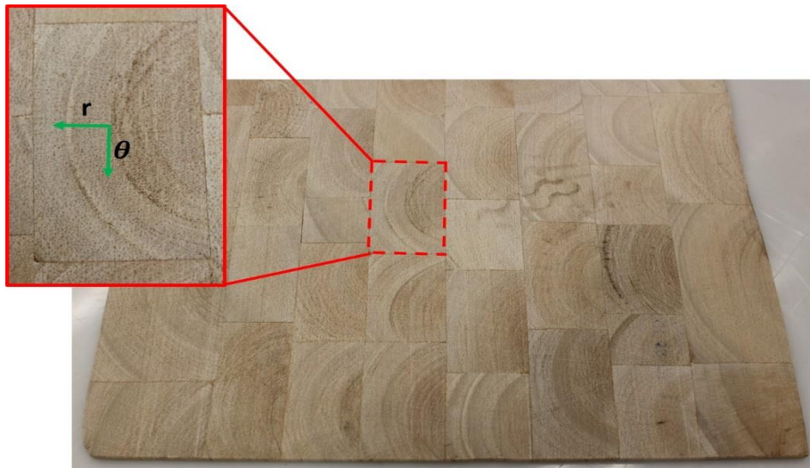
Fig. 8. Balsa core sheet shown with individual region highlighted. Note that each region can be described by a (r,\theta,z) system and that the bonded surfaces are clearly visible between any two regions.
