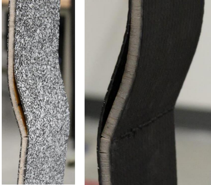
Fig. 65. Post-buckling failure of sample D2-4 with a 6.35 mm thick core.
