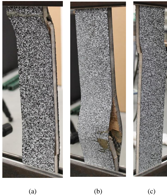
Fig. 46. Global failure modes observed for test articles with no debond. (a) ND4-1 (L = 584 mm), (b) ND4-4 (L = 582 mm), (c) ND7-6 (L = 709 mm).
