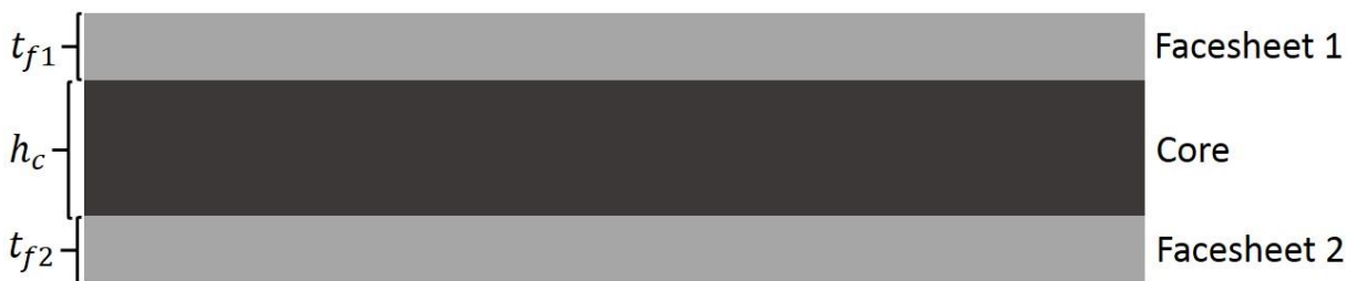
Fig. 1. Side view of sandwich composite construction. Facesheets do not have to be composed of the same material or thickness.
