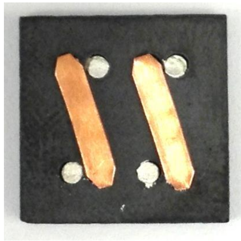
Fig. 3.19. Fabricated lateral flux coupled inductor substrate for 4 MHz POL module.
