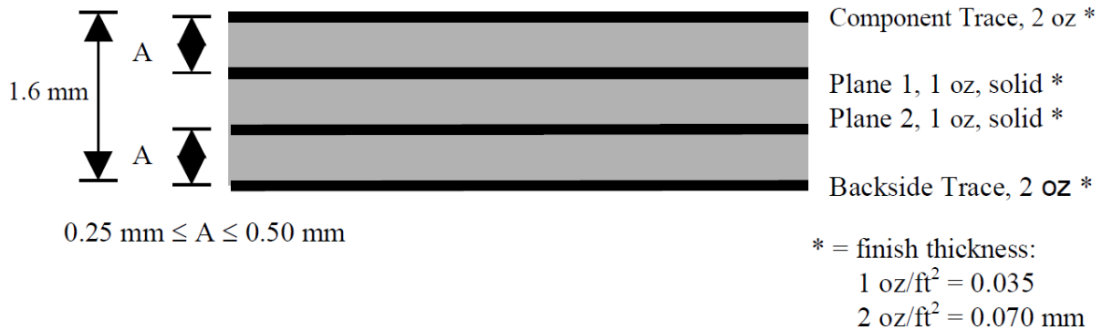
Fig. 4.21. Cross section of multi-layer evaluation board showing PCB trace and dielectric thicknesses [83].
