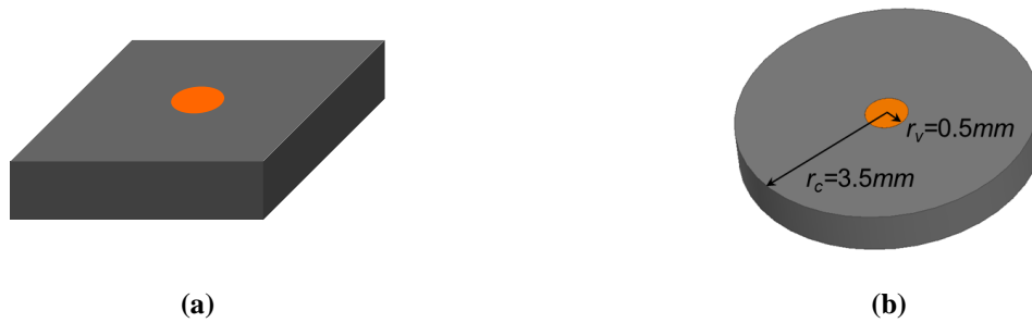
Fig. 6.1. Half core of the single-turn lateral flux inductor: (a) unit cell in square, (b) disc core in circle.
