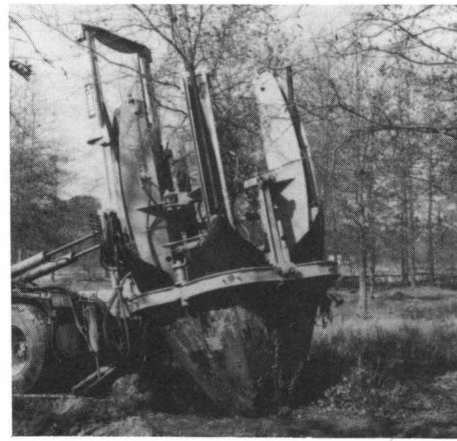
Mechanical tree digger removing a large shade tree. The planting hole at the landscape site has been pre-dug. This allows tree to be handled without burlapping and tying. (Greenbrier Farms, Chesapeake, VA)
