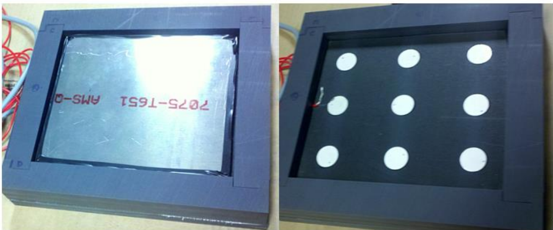
Figure 48. Photo. The energy harvester following the concept of AD5 (left) with aluminum cover, (right) without aluminum cover.
