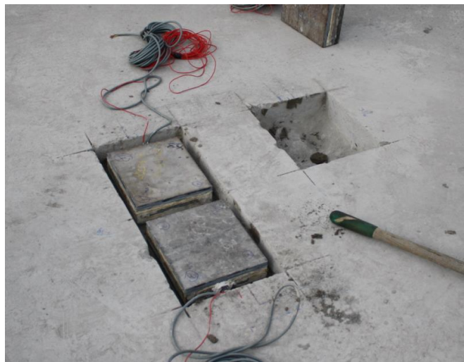
Figure 126. Photo. Applying a thin layer of epoxy in the prepared pits (to have a good bonding).
