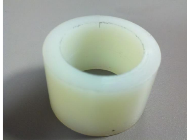
Figure 20. Photo. Nylon protective wall.
