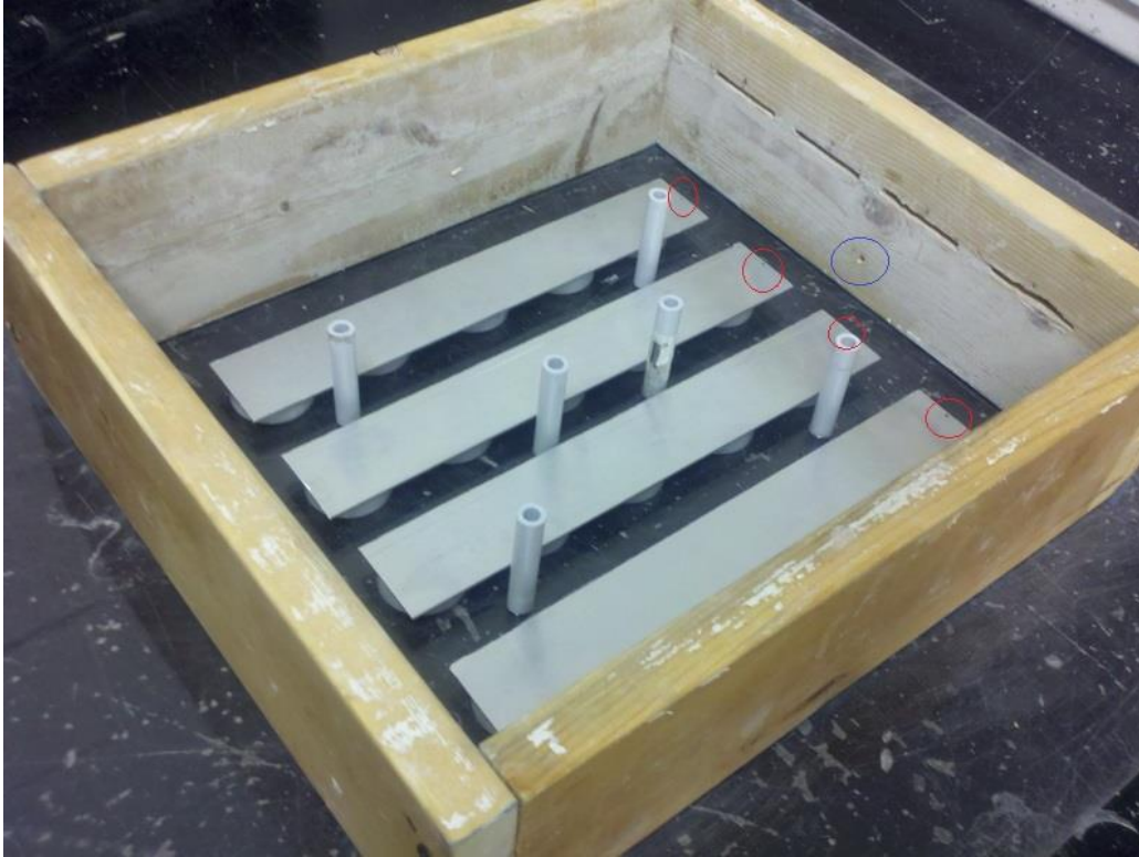
Figure 38. Photo. The assembled mold without electric wires.
