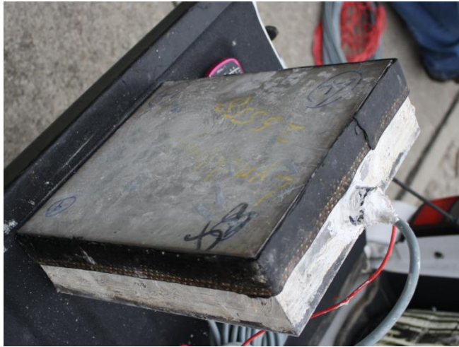
Figure 125. Photo. Wrapping the sides of energy harvester with rubber membrane.
