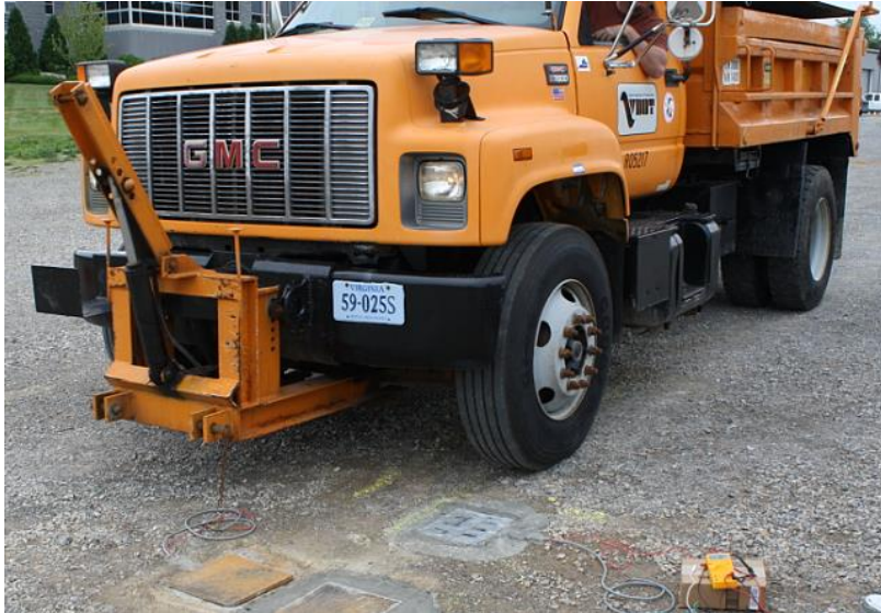
Figure 91. Photo. The dumper truck used to test the electric performance.
