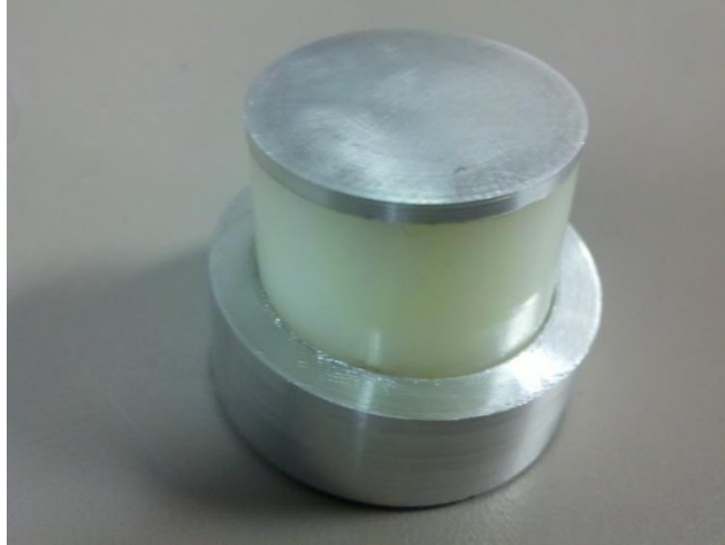
Figure 23. Photo. Assembled proto type piezoelectric energy harvester.
