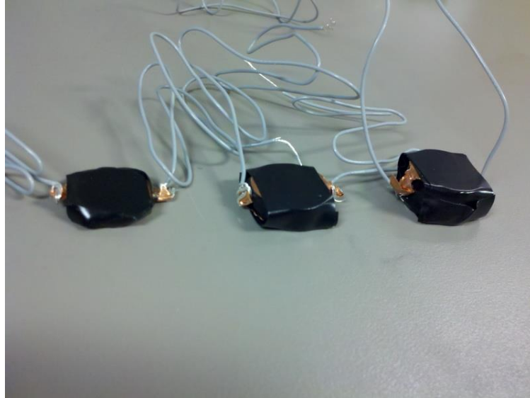
Figure 67. Photo. Piezoceramic disk specimens for simple preliminary tests (single-layer, tripple-layer and five-layers, from left to right).
