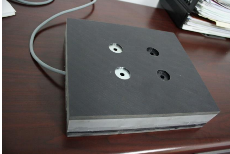
Figure 60. Photo. The energyharvester fabricated following AD7 (assembled).
