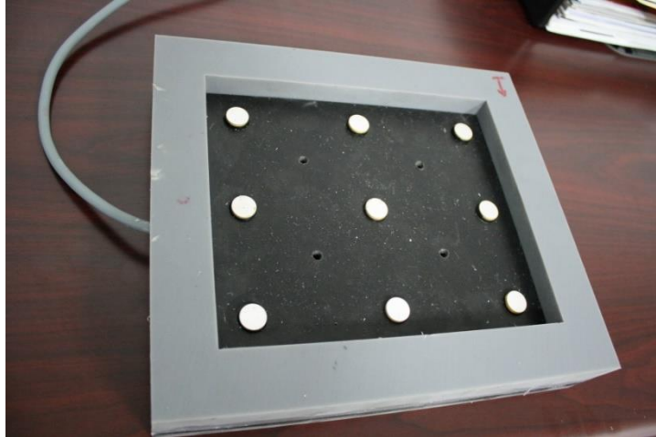
Figure 58. Photo. The energy harvester fabricated following AD7 (without cover).
