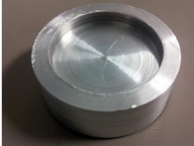
Figure 21. Photo. Aluminum alloy base with circular notch.
