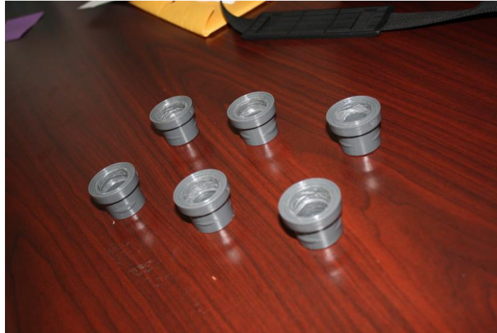
Figure 61. Photo. The candidate flange for protecting the cable exit in the Trouville installation.
