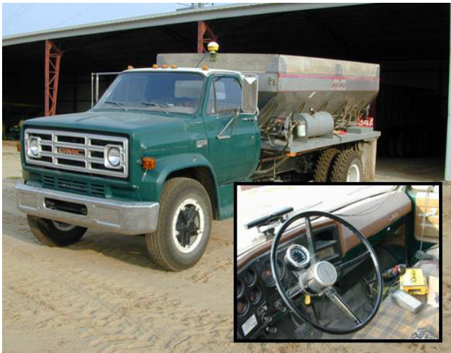
Figure 3. GPS navigation system mounted in a spinner spreader.
