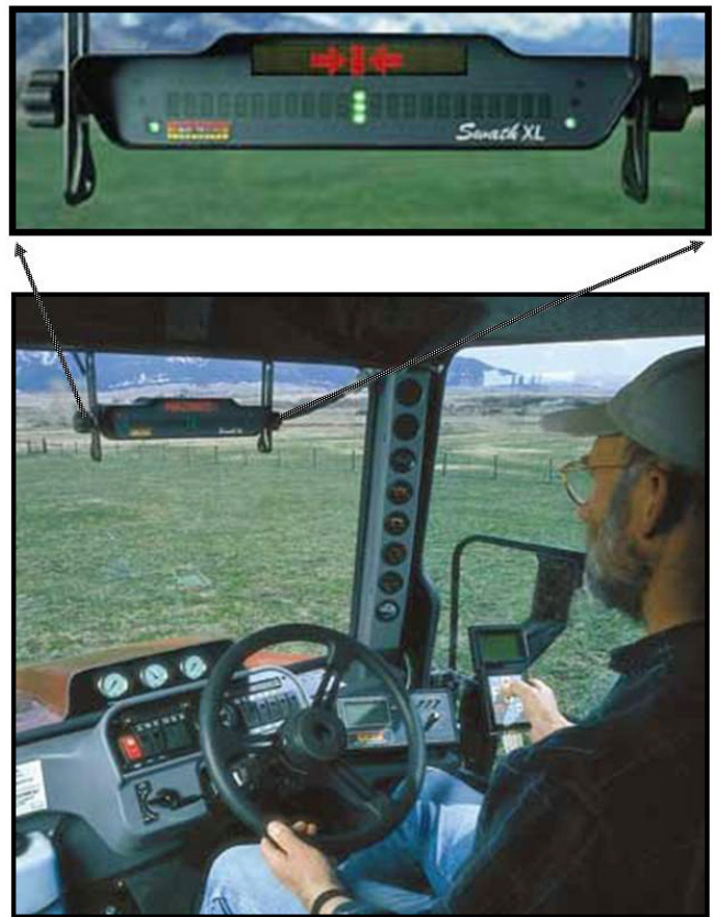
Figure 1. Lightbar navigation system mounted in cab and in view of forward travel.
