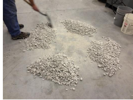
Figure 18. Sampling the aggregates by quartering method
