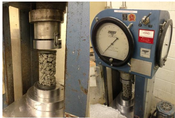
Figure 60. The compressive strength test on OGPCCB-OK specimen
