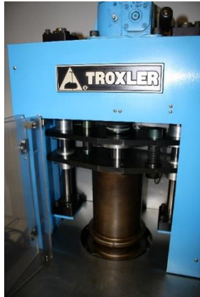
Figure 14. Using the Superpave Gyrotory Compactor (SGC) to compact specimens
