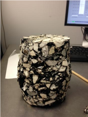
Figure 43. Largely deformed specimen under traditional stress levels
