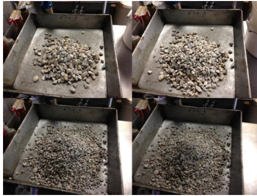
Figure 12. Adding aggregates of different sizes to produce ATPB-ID mixture
