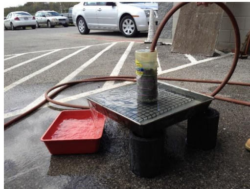
Figure 39. Apparatus for constant-head permeability test
