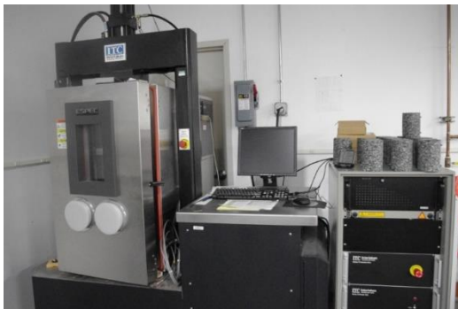
Figure 57. Apparatus for conducting the modified dynamic modulus test
