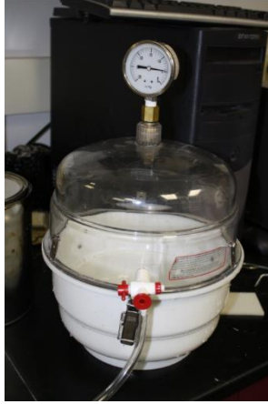
Figure 41. Setup for specimen saturation
