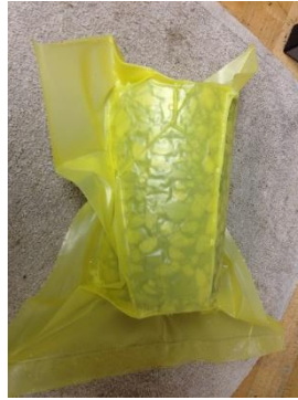
Figure 33. Sealed and vacuumed specimen
