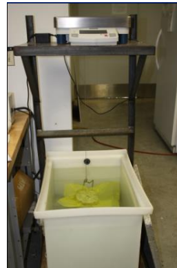
Figure 35. Water displacement measurement of sealed specimen
