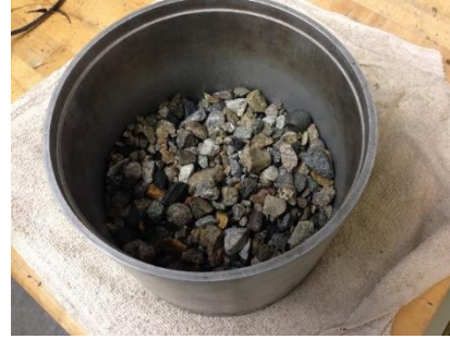
Figure 27. The Saturated Surface Dry (SSD) state of the unbound aggregates from ID
