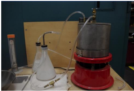
Figure 30. Vacuum the aggregates in water in a bowl
