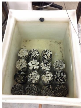
Figure 91. Submerged specimens in water tank for conditioning
