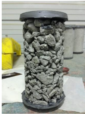
Figure 59. The capped OGPCCB-OK specimen
