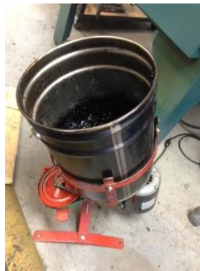
Figure 11. ATPB production for Idaho using drum mixer
