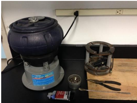
Figure 55. Apparatus for attaching aluminum studs on specimens
