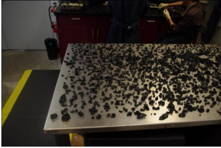
Figure 28. Separation of coated aggregates
