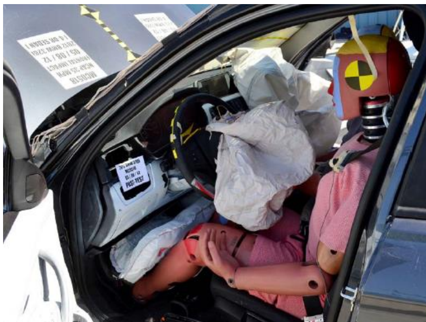
Figure 40. 2012 BMW 328i – NCAP Test 7857 Post-Crash Test Photo Showing Deployed Knee Airbag
