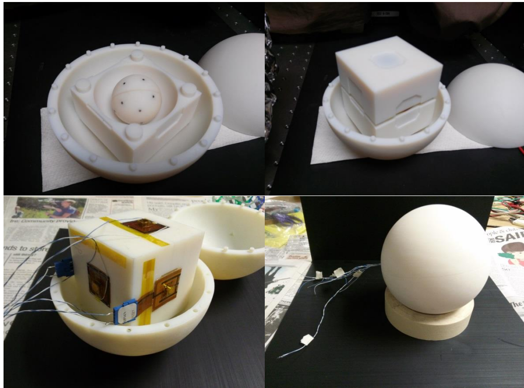
Figure 10.1 Ball Harvester concept using PiezoCap technology
