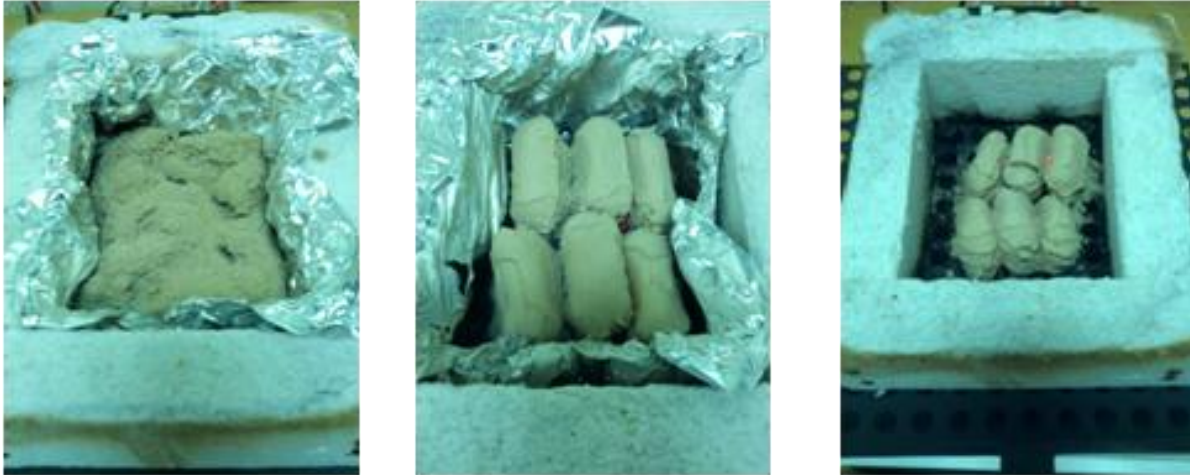
Figure 47: After-combustion three types of test conditions using EC fuel (a) Raw fuel in Al foil (b) Briquettes in Al foil (c) Briquettes in open grate system
