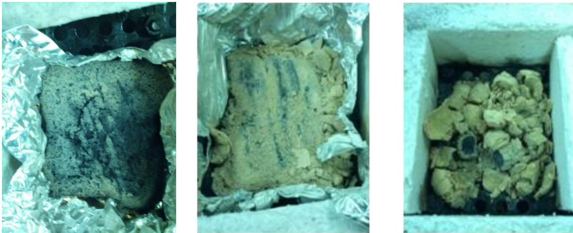
Figure 48: After-combustion three types of test conditions using EC fuel upon ash removal from upper surface (a) Raw fuel in Al foil (b) Briquettes in Al foil (c) Briquettes in open grate system
