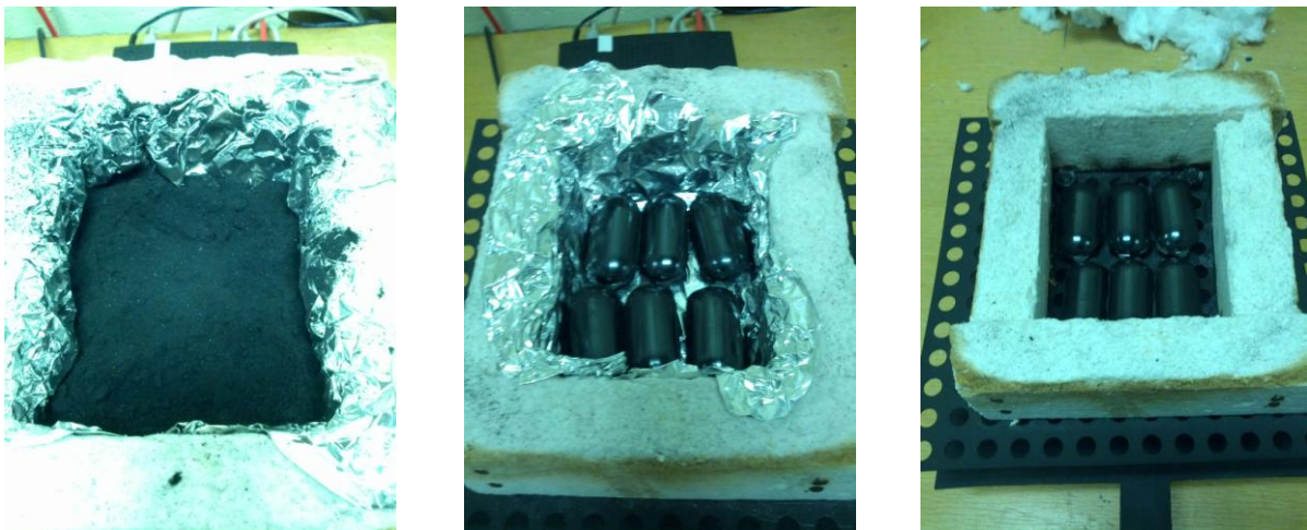
Figure 46: Three types of test conditions using EC fuel (a) Raw fuel in Al foil (b) Briquettes in Al foil (c) Briquettes in open grate system
