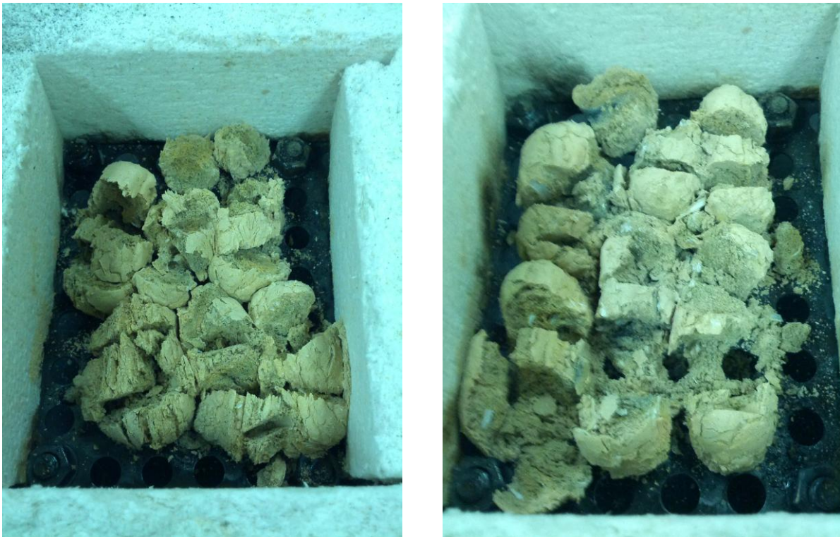
Figure 49: After-combustion two types of test conditions using blend briquettes upon ash removal (a) EC and SG-Raw briquette (b) EC and CS-Raw briquette
