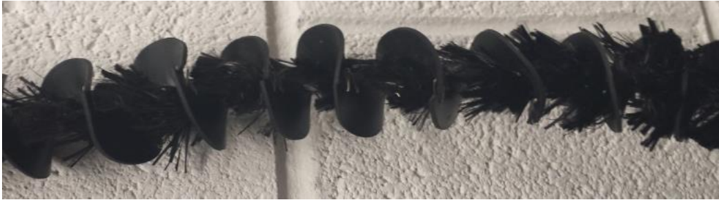
Figure 4.2: Photograph of the spiral spacer removed from the reaction chamber.
