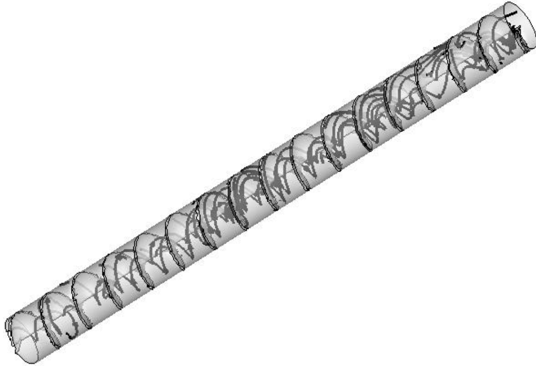
Figure 4.7: Streamlines of velocity magnitude for the reacting MFC system.
