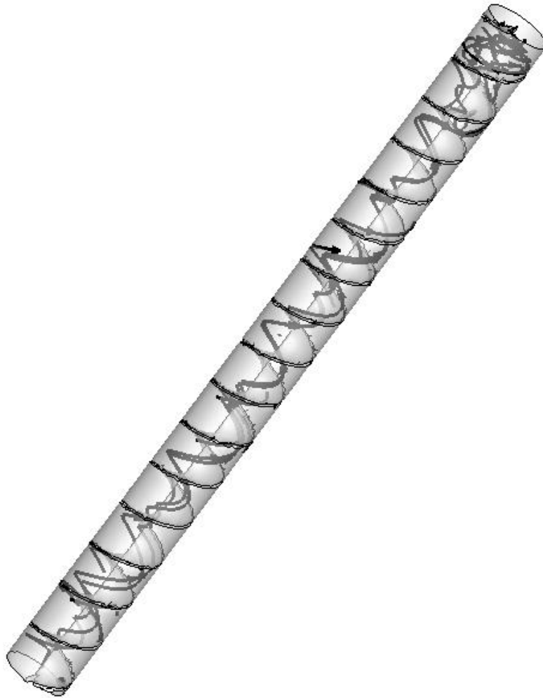
Figure 4.5: Streamlines of velocity magnitude for the non-reacting 3D MFC simulation.
