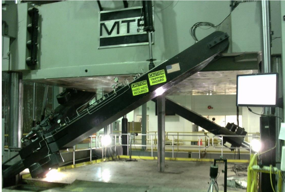
Figure 6.4: Standing support inside the MRS
