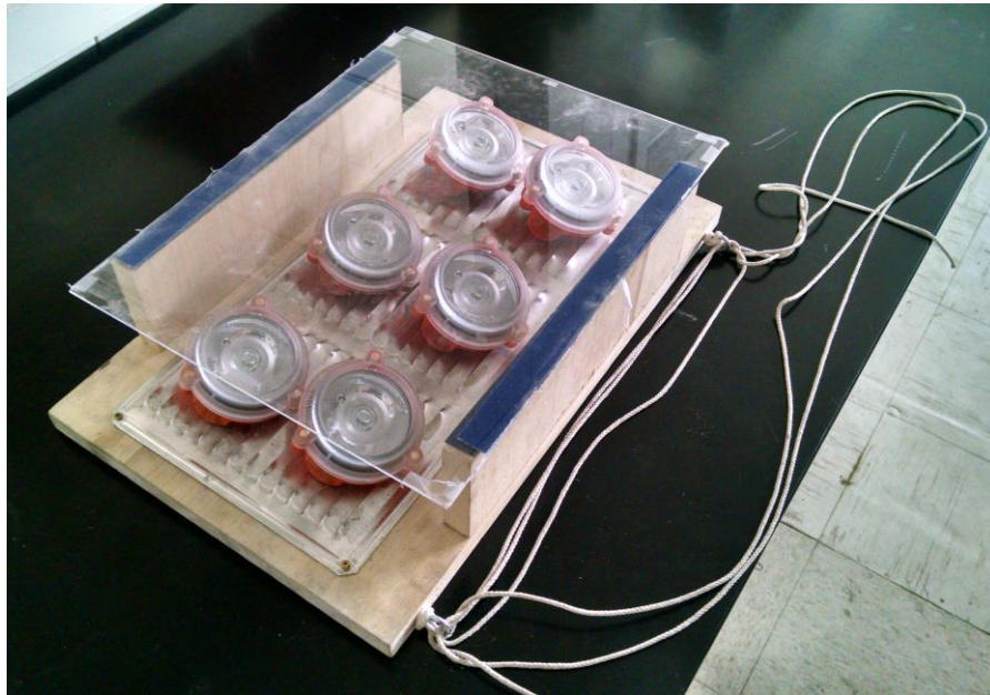
Figure 7.5: Mobile array of cap lamps for use in underground mine illumination
