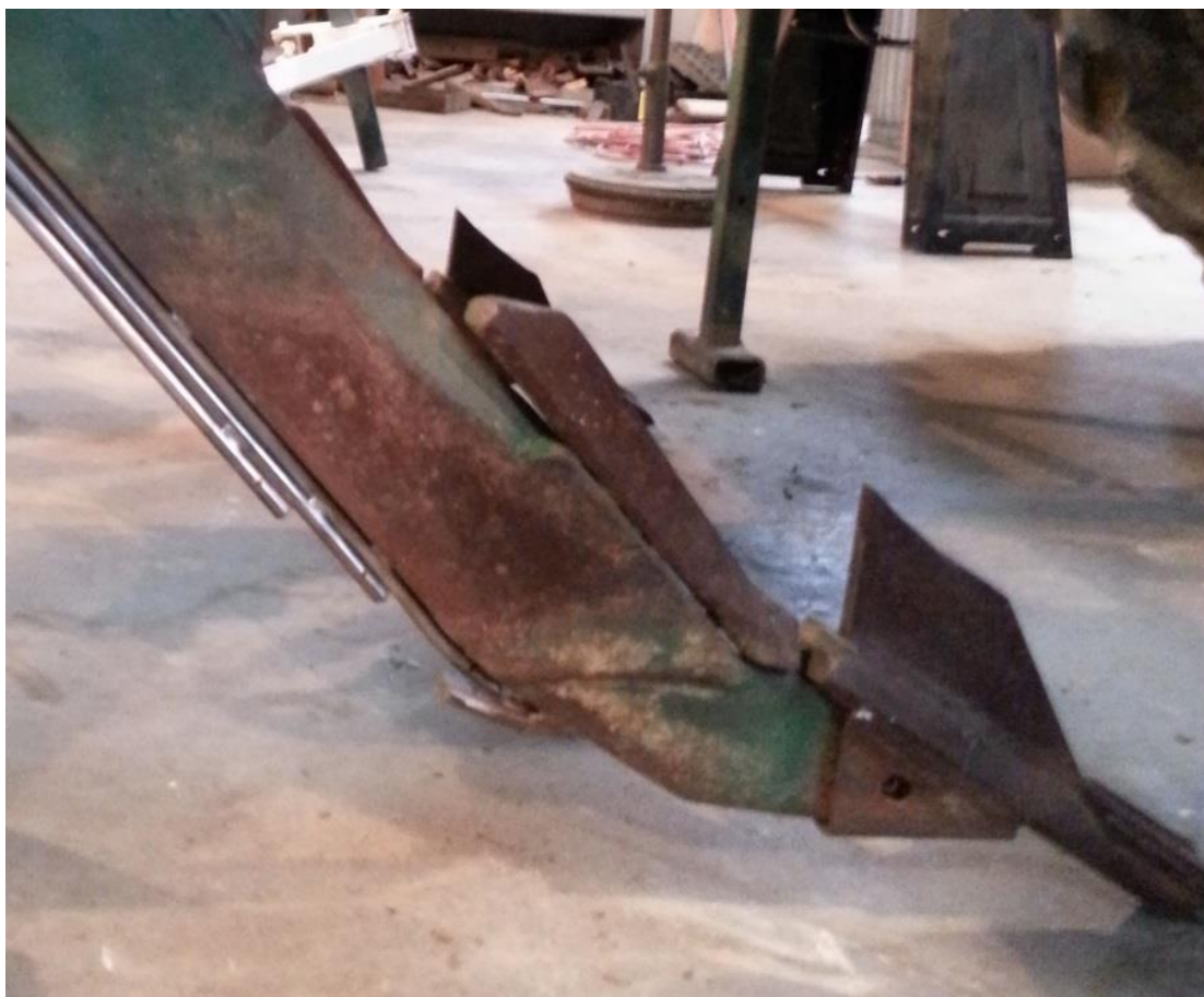
Fig. 3.1: Deep placement fluid fertilizer delivery system used in a P and K fertilizer rate and placement cotton study.
