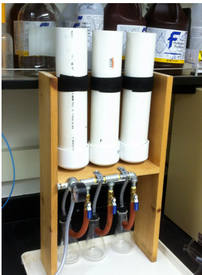
Figure 2. Image of vacuum column design used on treatment three columns. Pressure gauge used to insure vacuum set to -20 kpa (-0.2 bars).
