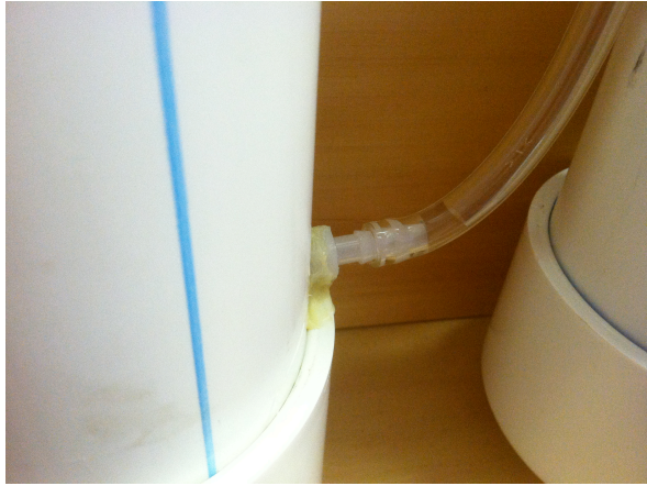
Figure 3. Visual confirmation of perching. This was the only occurrence of perching, as noted by the presence of leachate in the standpipe.
