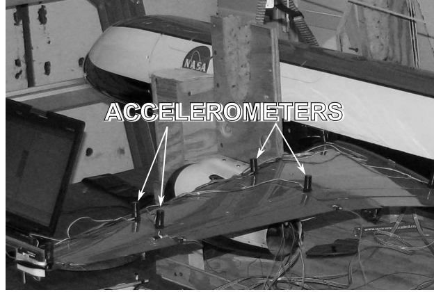
Figure 3.3: GVT Wing Accelerometers
