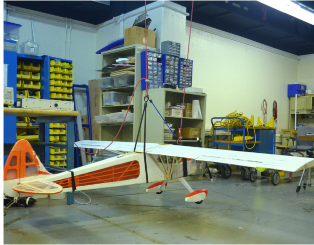
Figure 6.7: Suspension of Rascal for GVT
