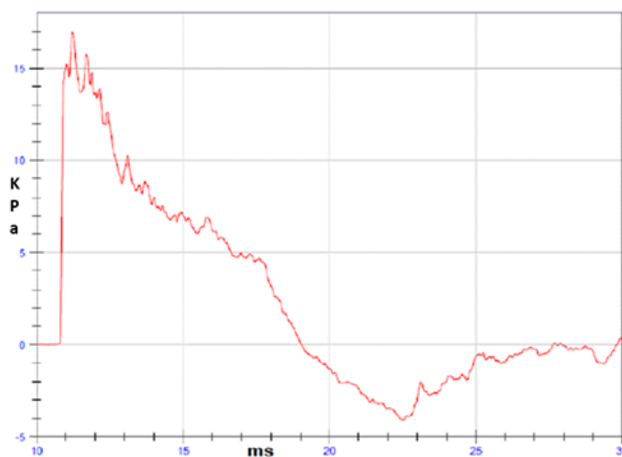
Figure 5.1: Representative pressure profile of calibrated shock wave to which animals are exposed with a resultant peak positive overpressure at 117 KPa
