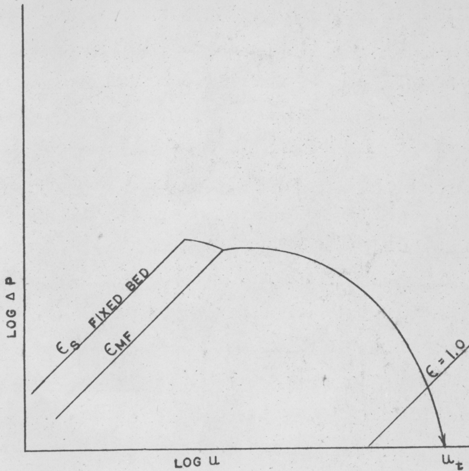
FIGURE 5. RELATION OF PRESSURE DROP TO FLUID VELOCITY IN A FLUIDIZED BED.
