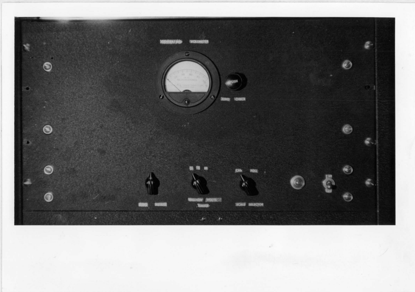
GENERATING VOLTMETER PANEL FIG. 10
