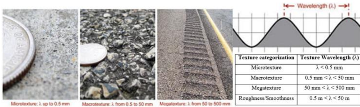
Figure 1-2 Physical representation of pavement texture (4; 5)
