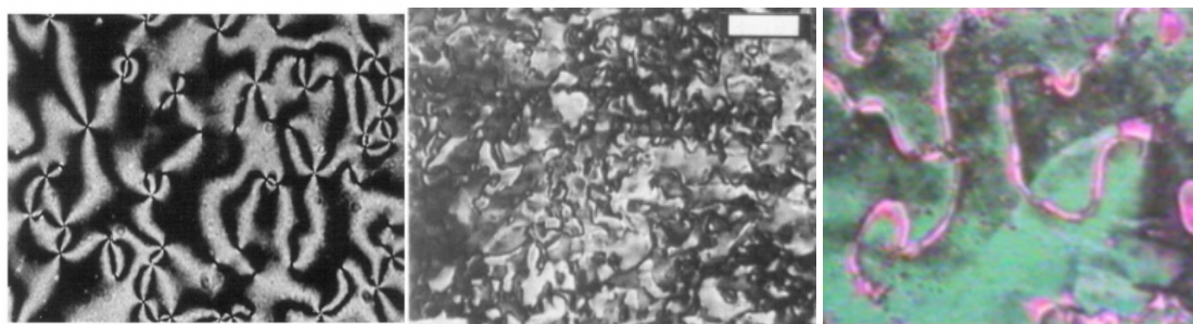
Figure 2.10: Various textures of nematic liquid crystals (a) Schlieren texture of 4-n-caproyloxy-4'-ethoxyazoxybenzene 40 (b)Marbled texture of Azo-benzene compound after uv exposure 41 (c)Thread like nematic LC texture of Benzoic Acid, 4-(4-Pentenyl-2-Methyl-1,4-phenylene Ester) 42
