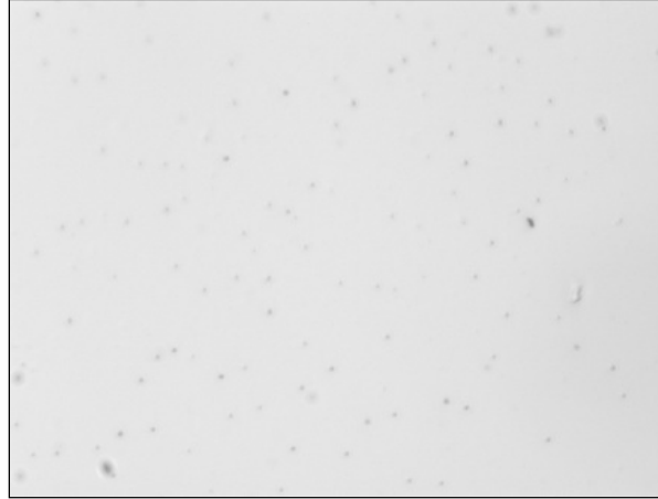
Figure 4.4: 55% 8CB fully dissolved in polysulfone, 175 °C
