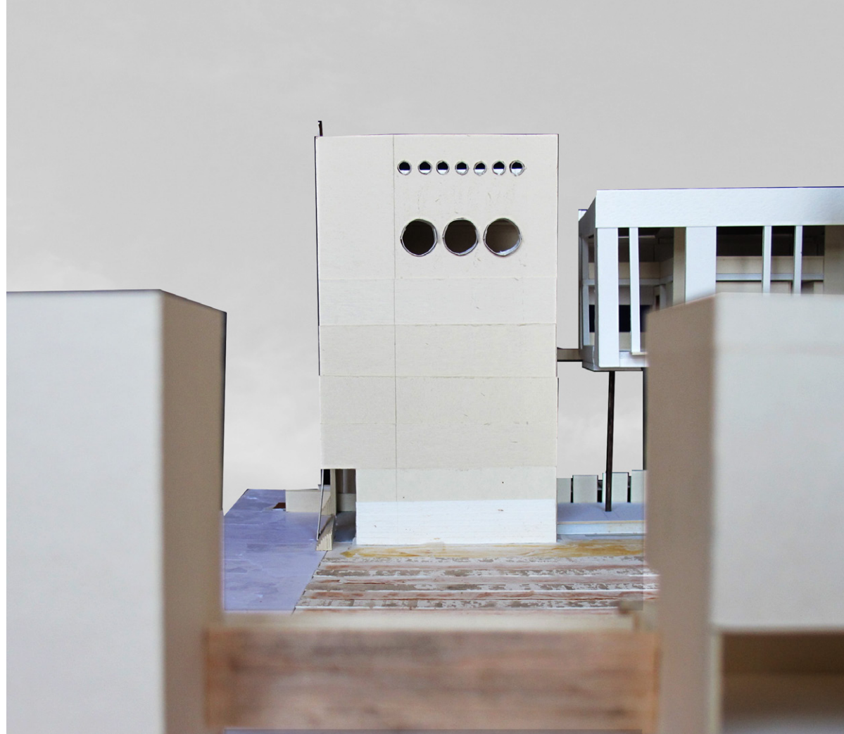
Final Model: looking from chef's house toward "pickled facade" - the wall weathers through the directed drainage of the wall.
