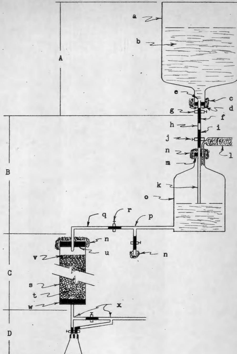
Figure 1 - Component Parts of the Pure Culture Experimental Tricking Filter
