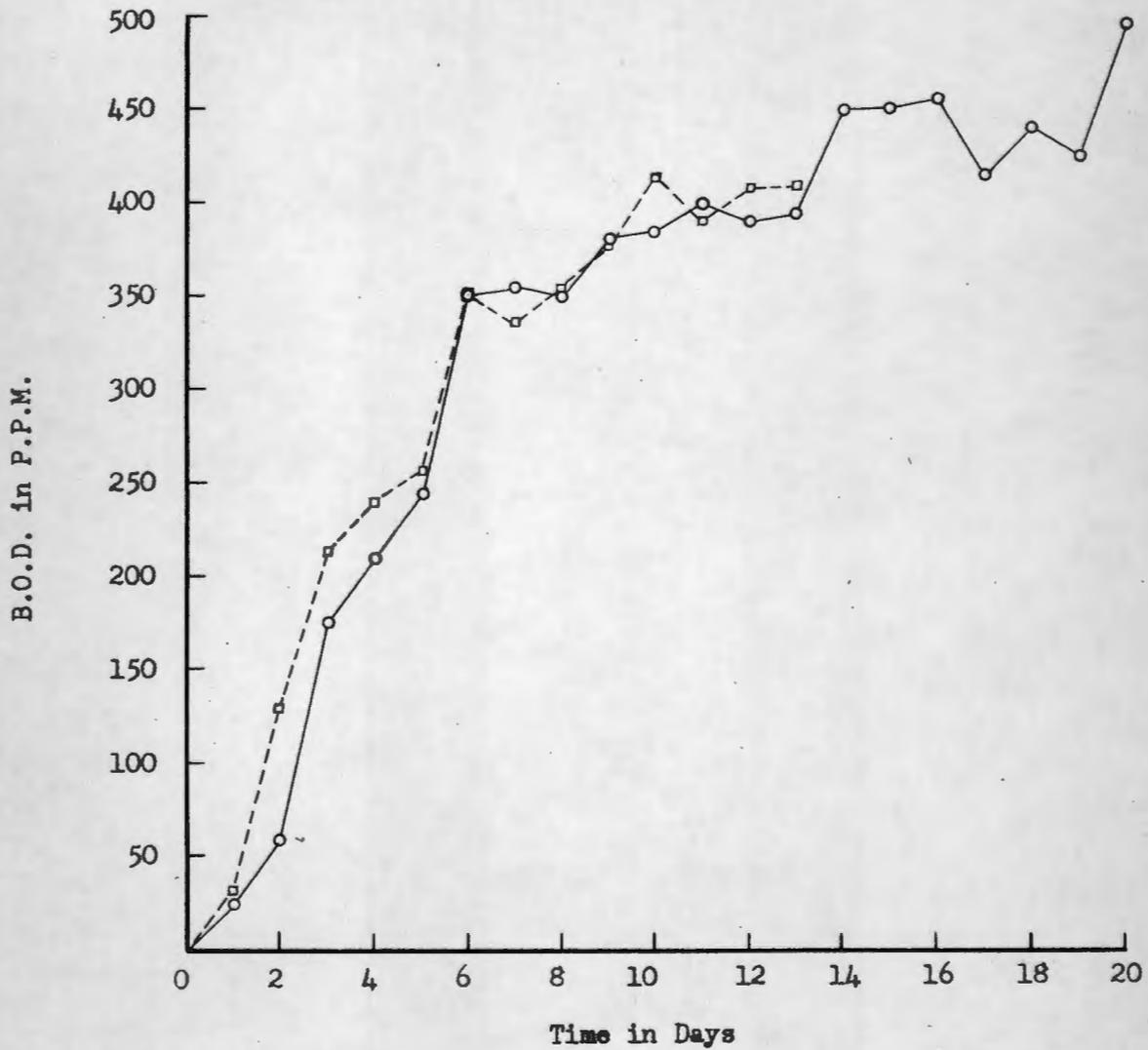
Figure 4 - Characteristic B.O.D. Curve for Synthetic Sewage
