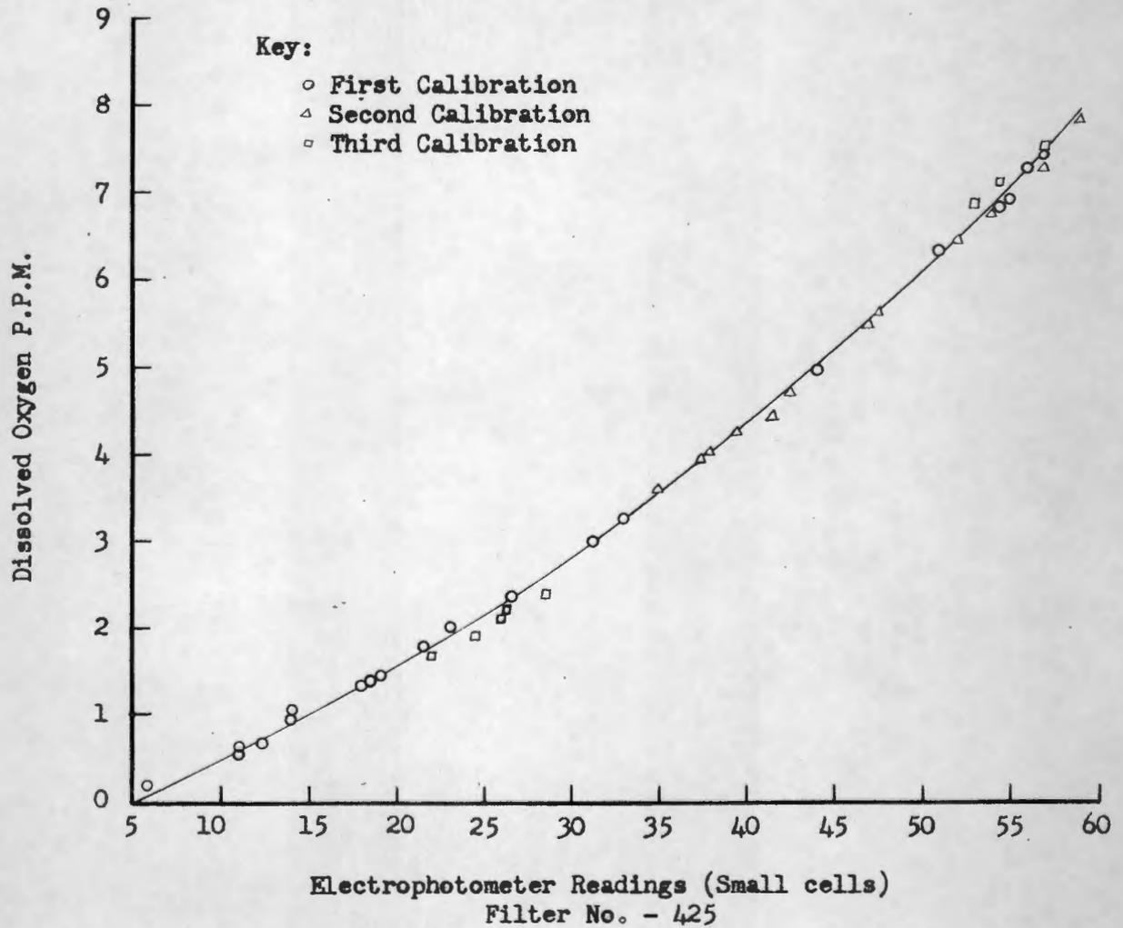
Figure 3 - Calibration Curve for Dissolved Oxygen Determinations by Electrophotometer Methods
