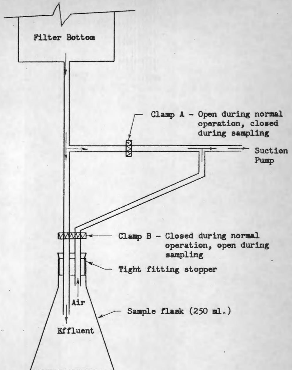
Figure 2 - Component Parts of the Filter Effluent Sampling and Disposal Set-up
