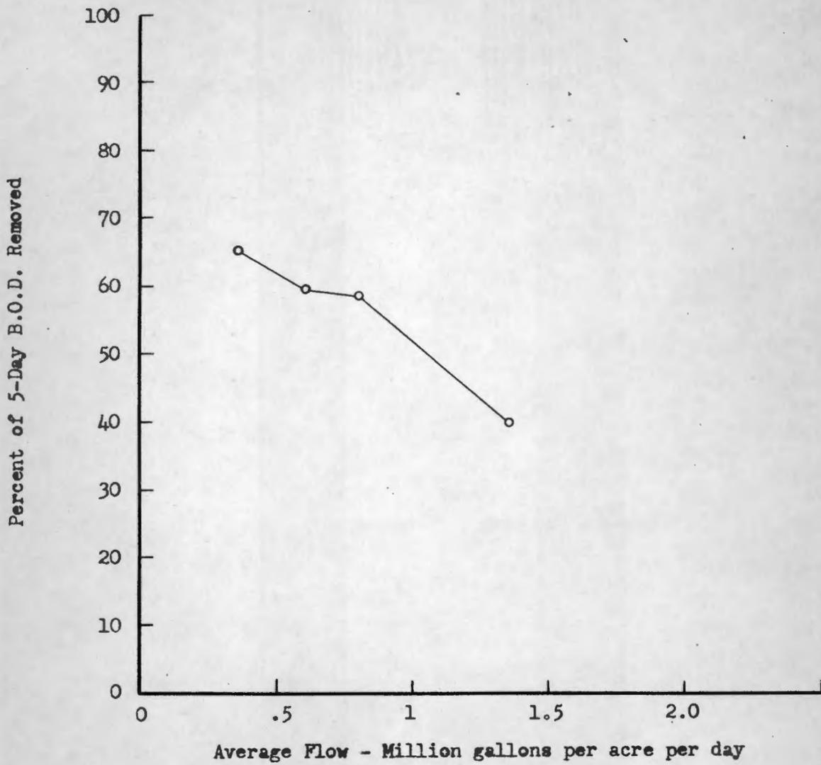
Figure 5 - Average Reduction in 5-Day B.O.D. of Synthetic Sewage by Zoogloea ramigera with Varying Rates of Flow
