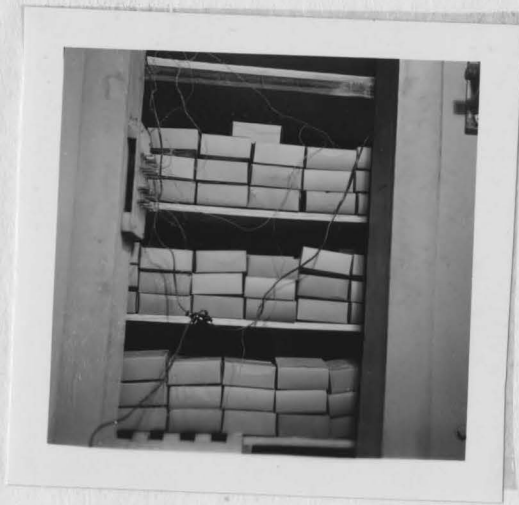
Figure 17 View of 554-pound Storage Load Used in Tests of SERIES D-4 .
