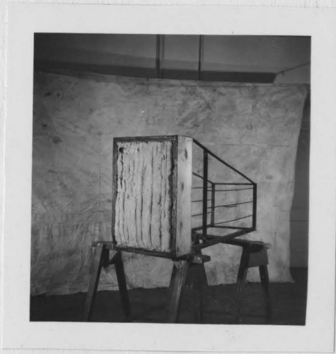
Figure 3 Insulation in Place Notes: Conduit in Upper Left.
