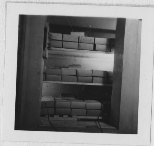
Figure 19 View of Storage Load on Shelves as Used in Tests of SERIES D-5 .
