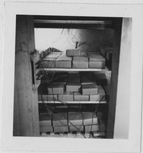
Figure 15 View of 277-pound Storage Load Used in Tests of SERIES D-3 .
