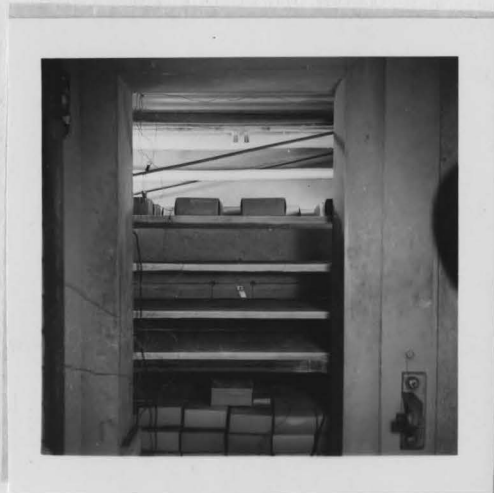
Figure 18 View of Evaporator Plates and Freezing Load at End of Tests in SERIES D-4 .
