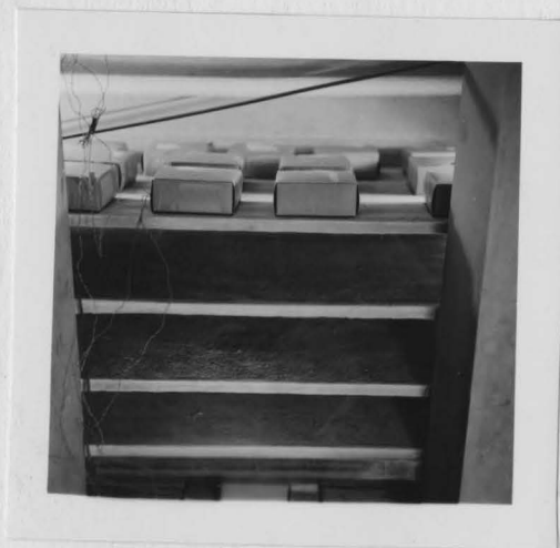
Figure 16 View of Evaporator Plates and Freezing Load at End of Tests in SERIES D-3 .
