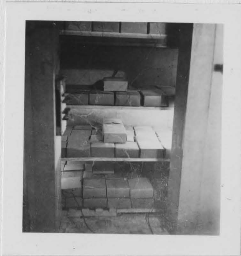
Figure 21 View of Storage Load on Shelves as Used in Tests of SERIES D-6 .
