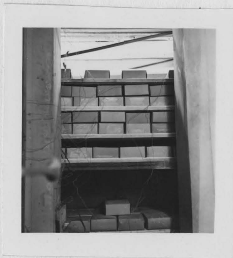
Figure 22 Evaporator Plates Showing Loading and Storage as Used in Tests of SERIES D-6 .
