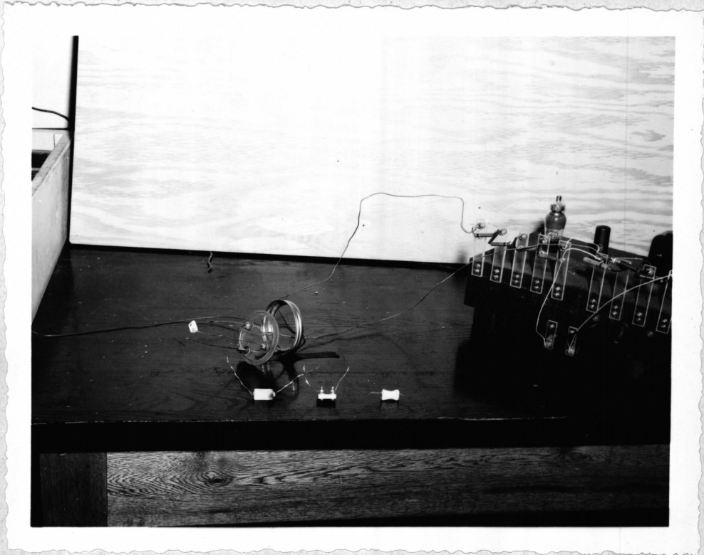
Figure 6. Vacuum Tube Voltmeter Connected to Element A through the Chamber Top Assembly. Element B is shown on the Left of two other Sample Elements
