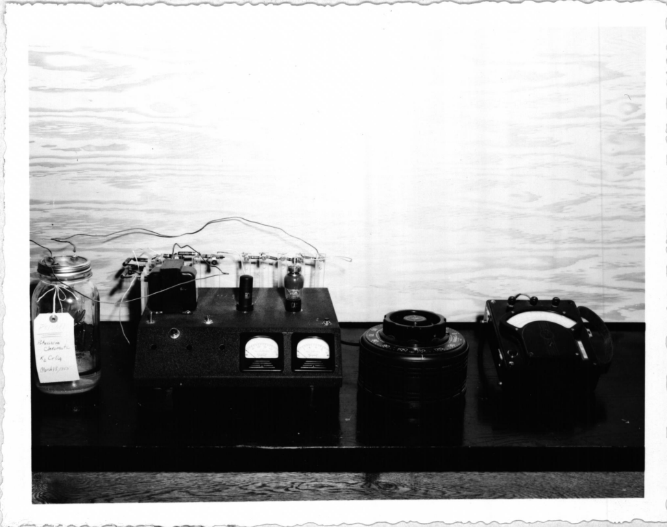
Figure 12. Reostat and Voltmeter Used to Maintain a Constant Input Voltage to the Vacuum Tube Voltmeter.
