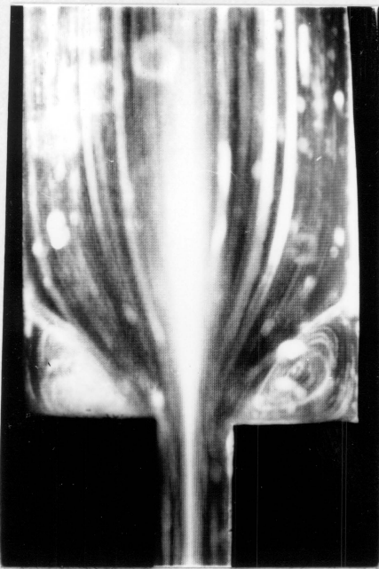
Figure 13. Streamline Patterns of LDPE, 4:1 Contraction: a) \dot{\gamma} = 20 \text{ sec}^{-1} , We = 1.29 b) \dot{\gamma} = 40 \text{ sec}^{-1} , We = 1.35 c) \dot{\gamma} = 60 \text{ sec}^{-1} , We = 1.38 d) \dot{\gamma} = 80 \text{ sec}^{-1} , We = 1.38
