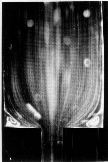
Figure 15. Streamline Patterns of Polystyrene, 4:1 Contraction, 190° C: a) \dot{\gamma} = 5 \text{ sec}^{-1} , We = 0.823 b) \dot{\gamma} = 20 \text{ sec}^{-1} , We = 1.19 c) \dot{\gamma} = 40 \text{ sec}^{-1} , We = 1.39 d) \dot{\gamma} = 80 \text{ sec}^{-1} , We = 1.62
