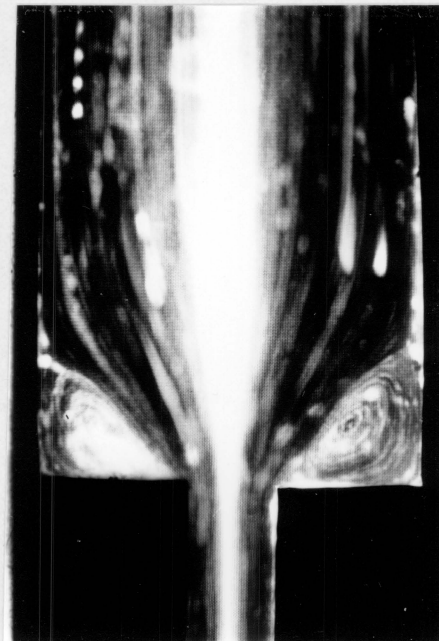
Figure 13. Streamline Patterns of LDPE, 4:1 Contraction: a) \dot{\gamma} = 20 \text{ sec}^{-1} , We = 1.29 b) \dot{\gamma} = 40 \text{ sec}^{-1} , We = 1.35 c) \dot{\gamma} = 60 \text{ sec}^{-1} , We = 1.38 d) \dot{\gamma} = 80 \text{ sec}^{-1} , We = 1.38
