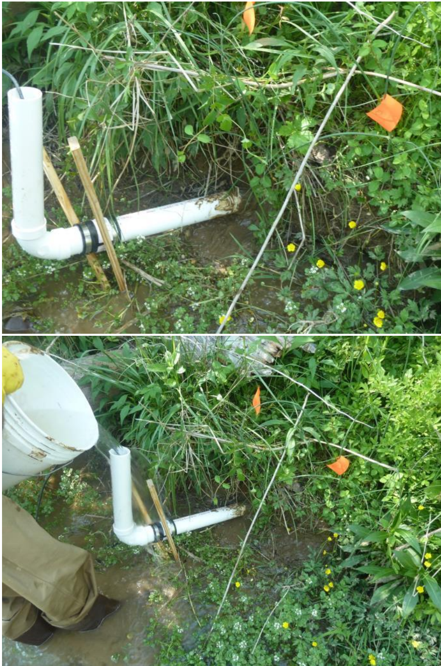
Figure E-2. Top panel shows apparatus set up inside macropore with a Leveltroll700 pressure transducer inside. Bottom panel shows the addition of water for a falling head test.
