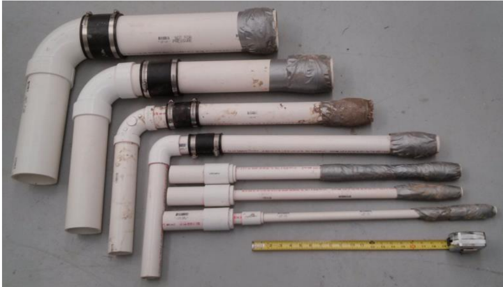
Figure D-1. Apparatuses to inject concrete into macropores. Ruler shows 0.5 m distance.
