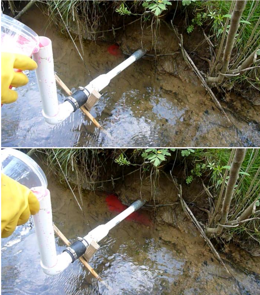
Figure E-1. Top panel shows tracer transport 10 seconds after rhodamine addition to apparatus installed in macropore. Bottom panel shows 30 seconds after initial addition of rhodamine.
