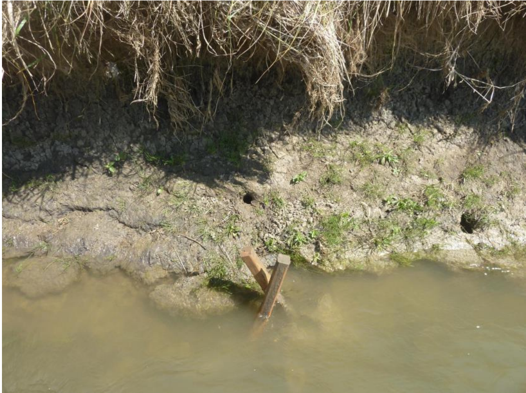
Figure D-2. Experimental macropore that extends 0.5 m into the bank.
