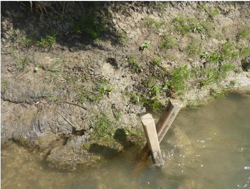
Figure D-5. Apparatus removed and macropore remains filled with hydraulic concrete.
