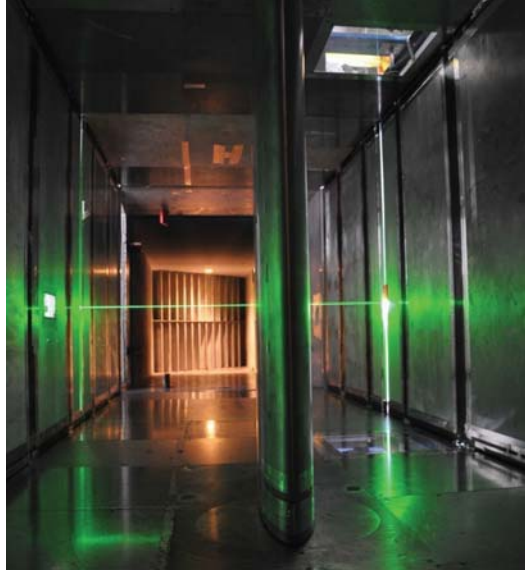
Fig. 3 Optical Wake Rake probe beam in the Stability Wind Tunnel downstream of the 0.800 meter DU96-W-180.
