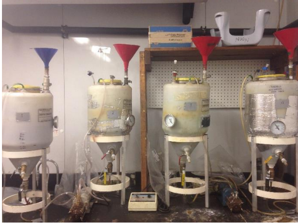
Figure 29 High-density polyethylene batch fermentation reactors supplied by the Hobby Beverage Equipment Company (Temecula, California)
