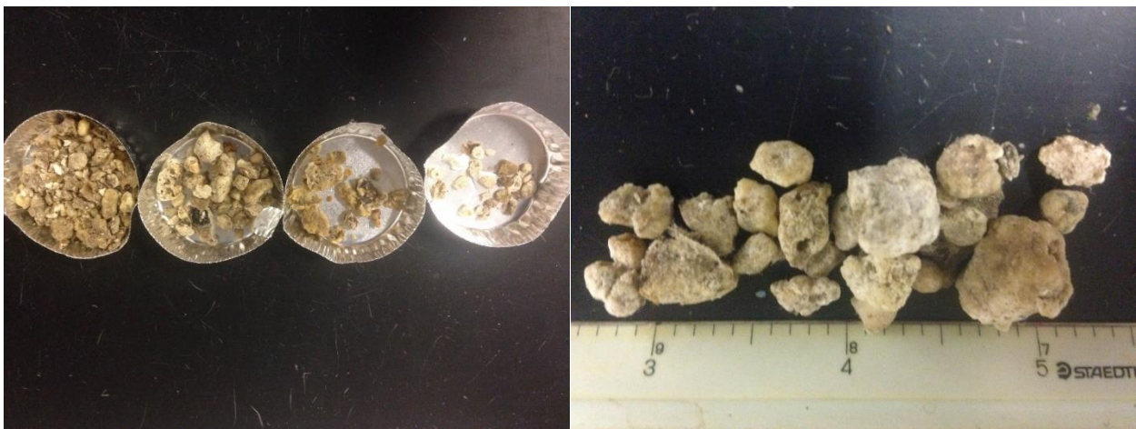
Figure 30 Accumulated LCFAs (grease balls) from the APDs during the 1st operating periods (left) and the grease balls (right) (ruler shown in inches)
