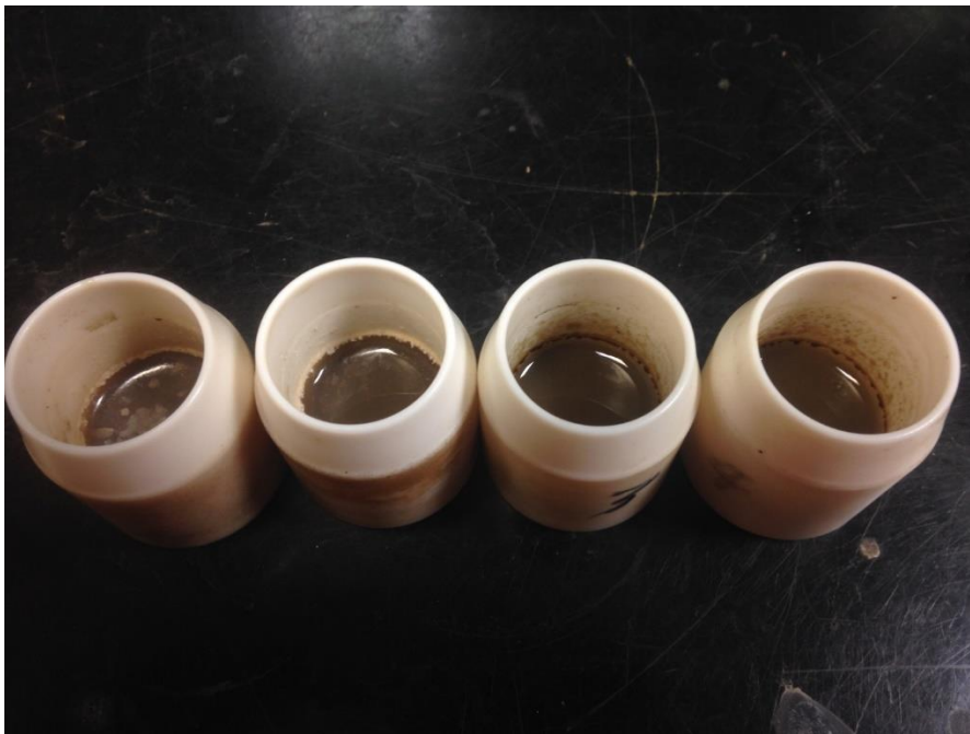
Figure 24 Thermal hydrolysis of LCFA with (10,000 mg/L COD) of digested sludge (8-hr thermal hydrolysis)
