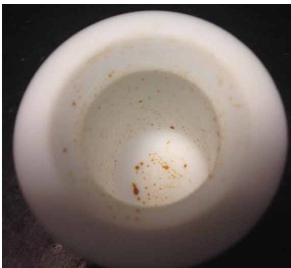
Figure 22 Unsaturated residuals after 8-hr thermal hydrolysis treatment
