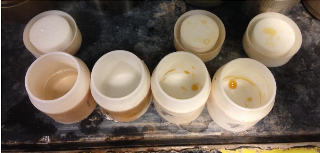
Figure 23 LCFA residuals after 8-hr thermal hydrolysis treatments: C16:0, C18:0, C18:1, and C18:2 (from left to right)
