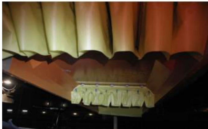
Figure 2: Underside of T-Craft model with seals in Bishop [2].
