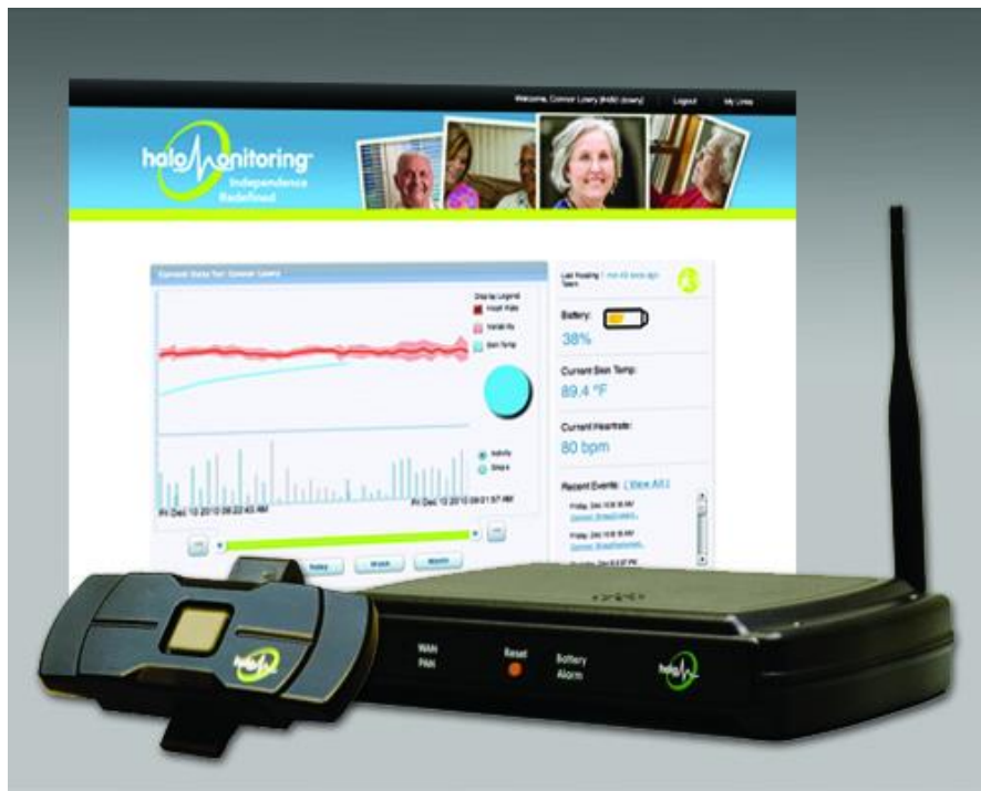
Figure 4.8: myHalo monitoring and home base device used to detect a fall [Online]. Available:
