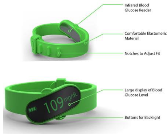
Figure 4.13: Sleep Well conceptual medical device used to check blood sugar in kids
