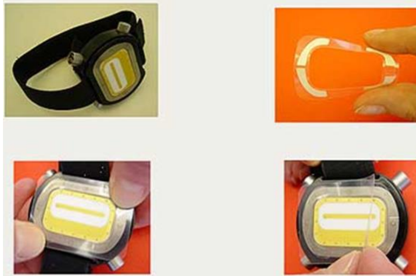
Figure 2.18: The adhesive tape for the Pendra used to detect the blood glucose
