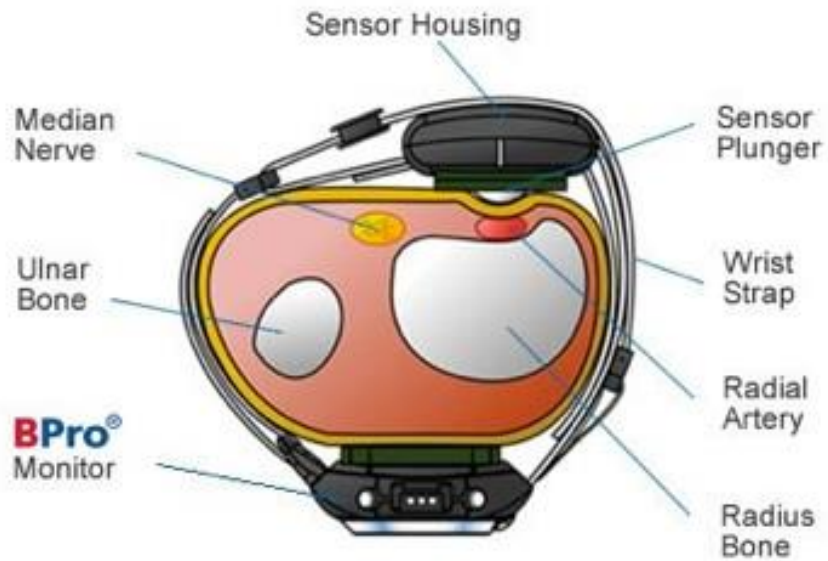
Figure 4.10: BPro medical device and its components used to monitor and detect stroke [Online]. Available: http://www.healthstats.com/index3.php?page=homepage . [Accessed 9 September 2013] Used under fair use, 2014
