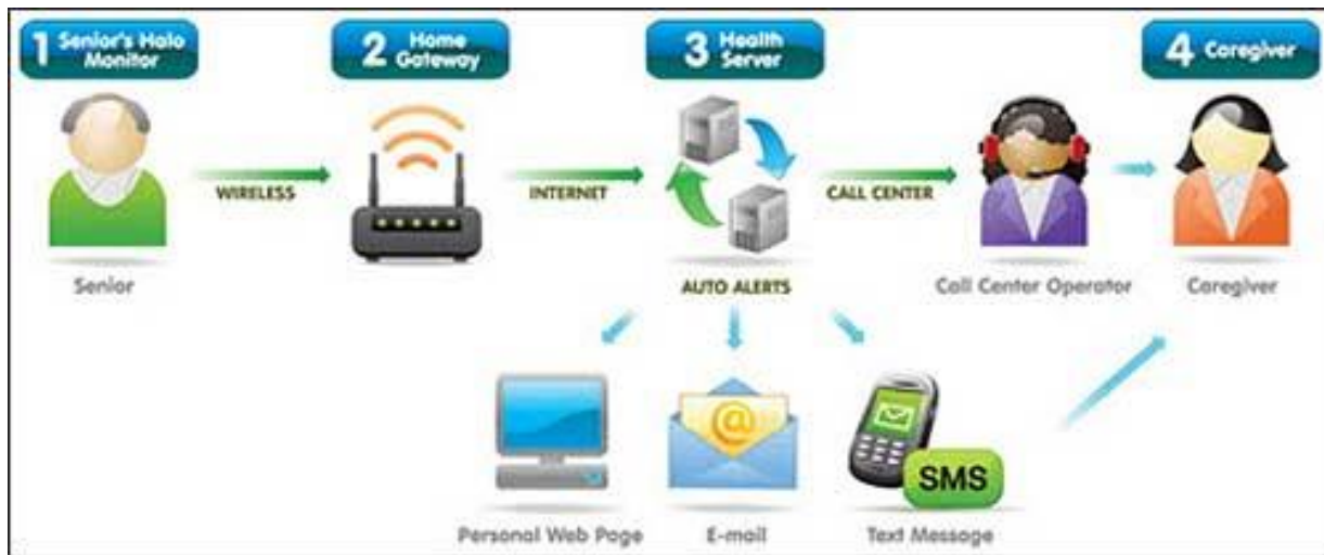
Figure 4.7: How myHalo works and communicates when an alert is signaled [Online]. Available:
