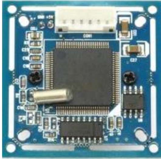
Figure 5.9: VC0706 UART Camera circuitry
